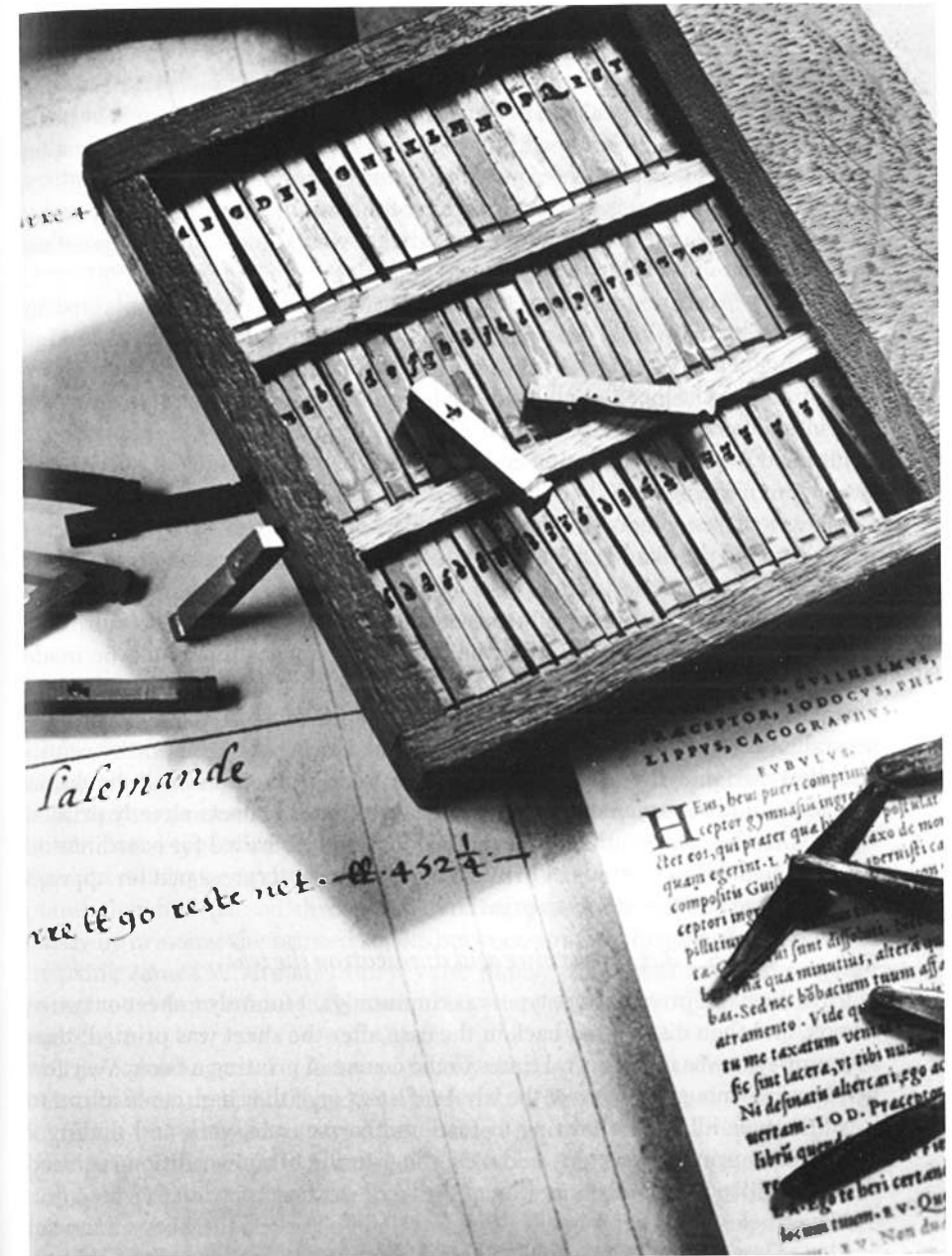
A box of John Fell's pica italic matrices, with some steel punches for larger capitals beneath them. By permission of Oxford University Press
