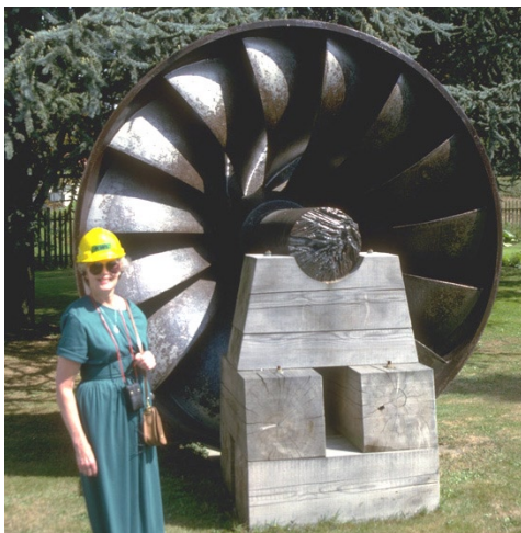
Fig. 11 - Typical Francis turbine rotor in use up to 1990. Fig. 12 - Textile industries in Lowell, Massachusetts grew based on available water power.
