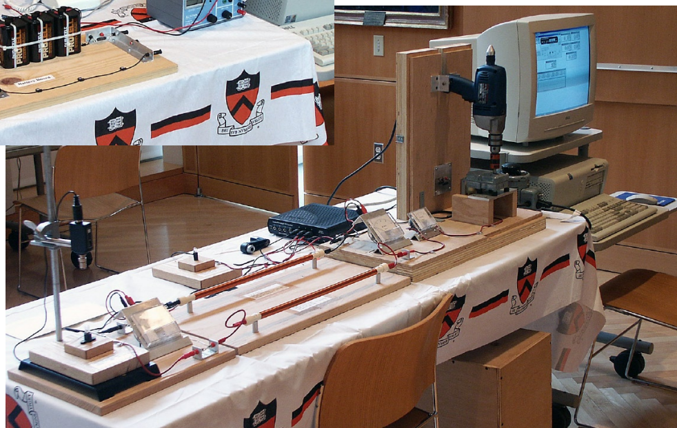
Fig. 2 - Experimental model of Edison's 1882 Pearl Street to Wall Street Lighting System.
