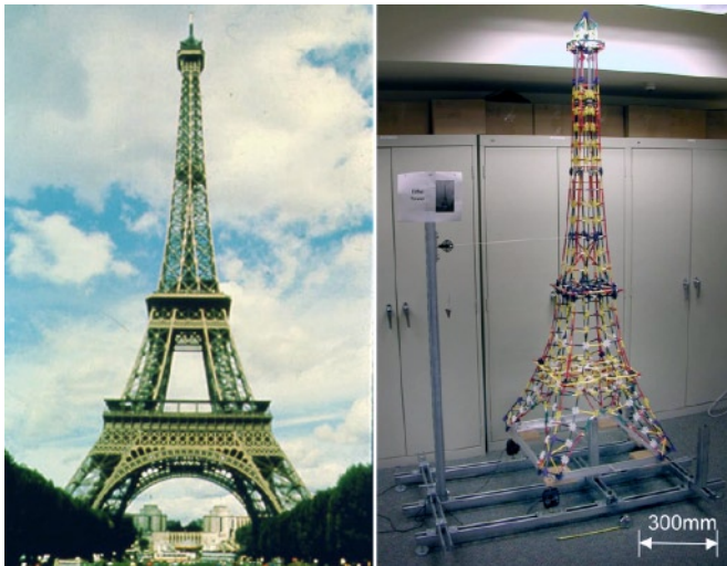
Fig. 2 - Eiffel tower and Eiffel tower model built from K'nex
