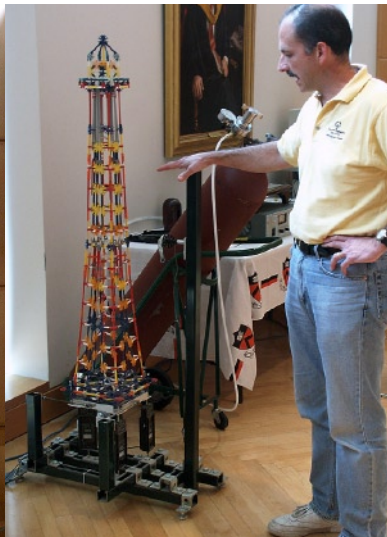
Fig. 3 - K'Nex model of the Eiffel Tower -- Used by students to understand free body diagrams and wind loading.
