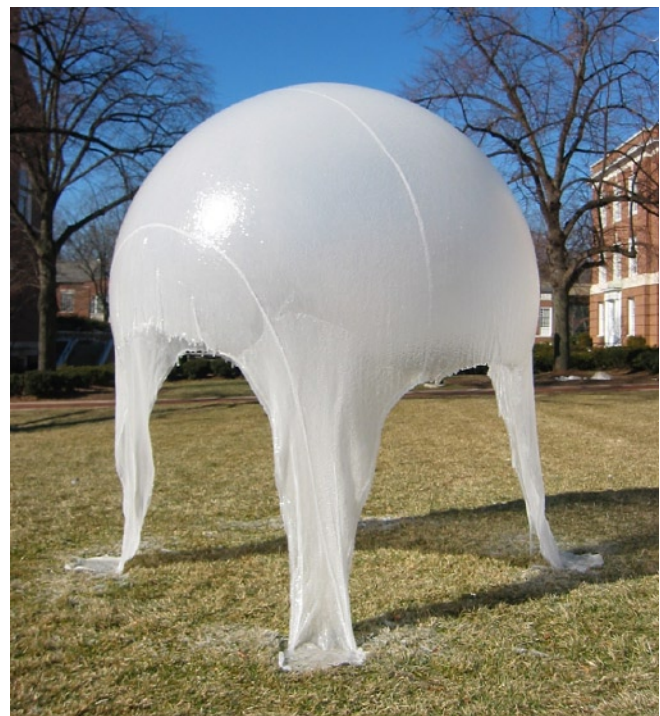
Fig. 3 - On a cold clear winter morning students on the Johns Hopkins campus were surprised to see this ice bubble sculpture created during a freezing night using a weather balloon and strips of cloth and water, demonstrating a concept shown in slides from Swiss engineer, Heinz Isler.
