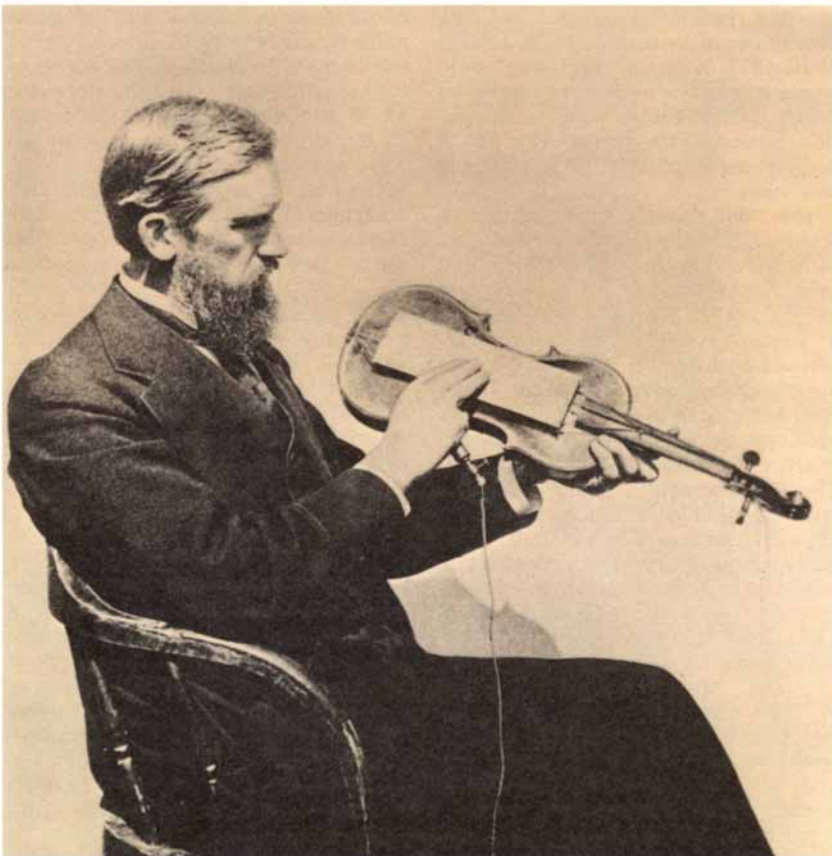
RECEIVING APPARATUS , a stringless violin with a silver plate covering the soundboard, was devised by Gray in 1874 to draw attention to the "vibratory currents" first made audible by the bathtub experiment (see top illustration on opposite page). Here one lead from the induction coil connects to the silver plate. The demonstrator (Gray in this instance) holds the other lead in his hand and rubs his fingers along the metal surface. The musical tone thus generated duplicated the tone of his transmitter, a metal reed that vibrated at audio frequencies.
