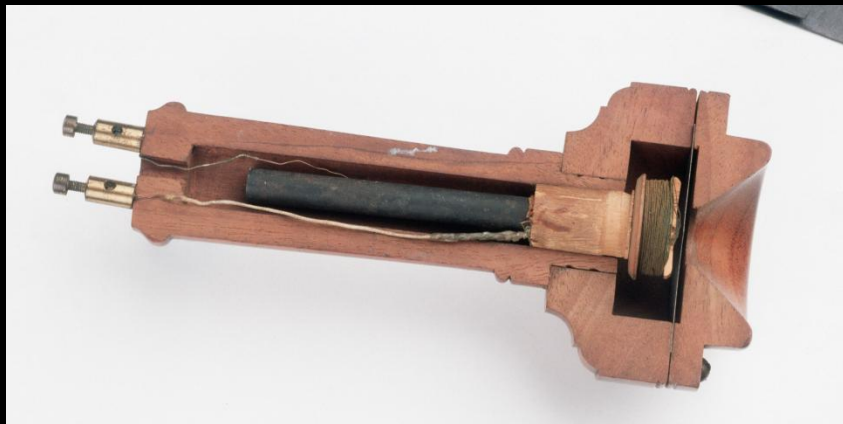
FIG. 62.—Cross-section of Bell Telephone Receiver.
