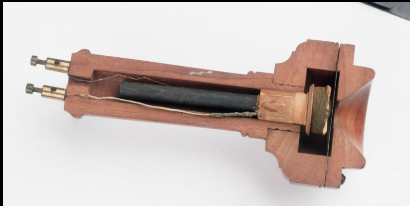
FIG. 62.—Cross-section of Bell Telephone Receiver.
