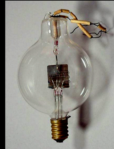
Light Bulb Triode as both One-Way Valve and Amplifier
