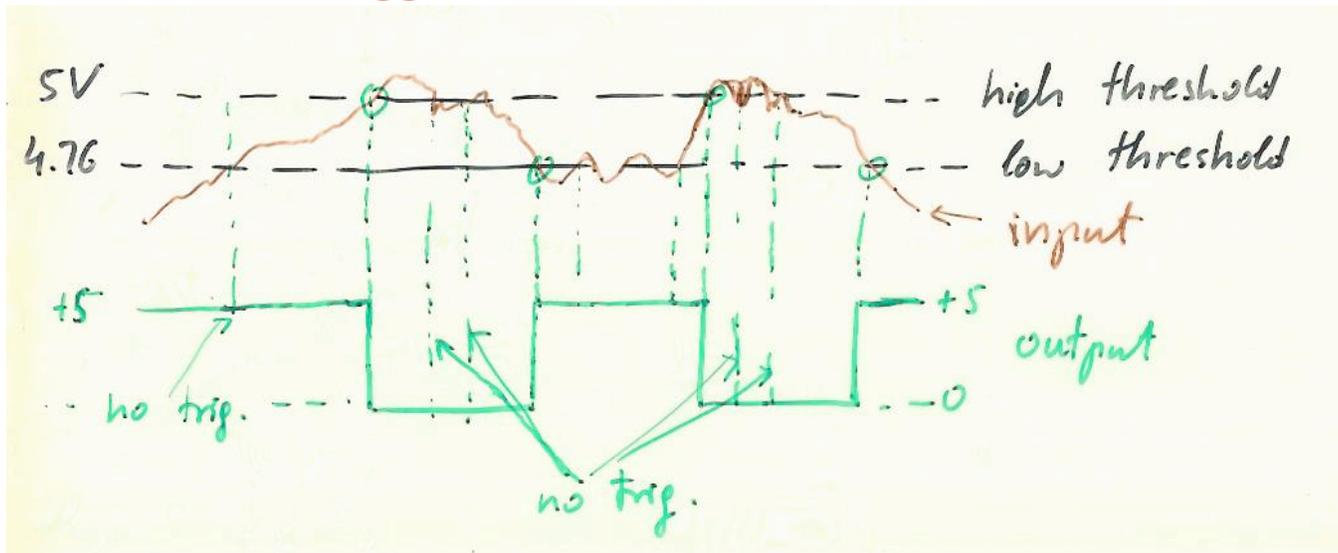
Resistance  $R_3$  (feedback) creates two thresholds, depending on the output state.
