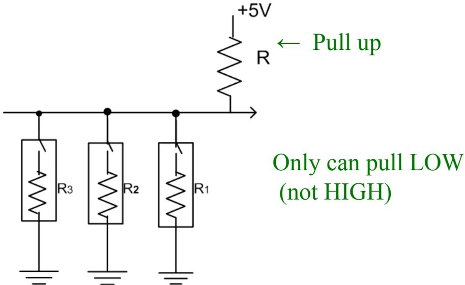
Open – Collector  $\Rightarrow$  doesn't have internal pull up  $\Rightarrow$  No HIGH
