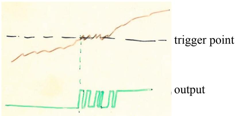
Solution: Positive feedback (Schmitt Trigger) which creates dual threshold.
