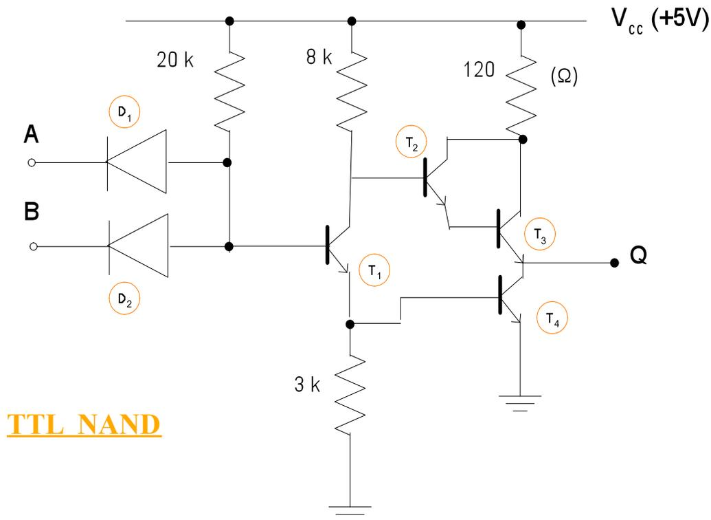
Analysis: Inputs A, B on diodes  $D_1$ ,  $D_2$  are driving transistor inverter followed by a push-pull output. If A and B are HIGH, the 20 kΩ resistor provides V for  $T_1$  to be “ON”,
