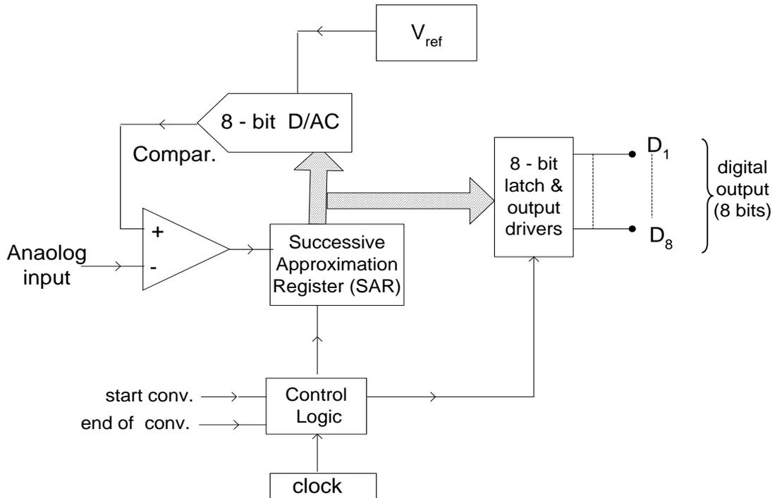
Start: all bits = 0 : MSB  $\Rightarrow$  1 and following bits  $\Rightarrow$  1. If D/AC output does not exceed the input voltage, this bit stays 1. Otherwise, it is set 0. For N – bit A/DC , N-such steps are required.
