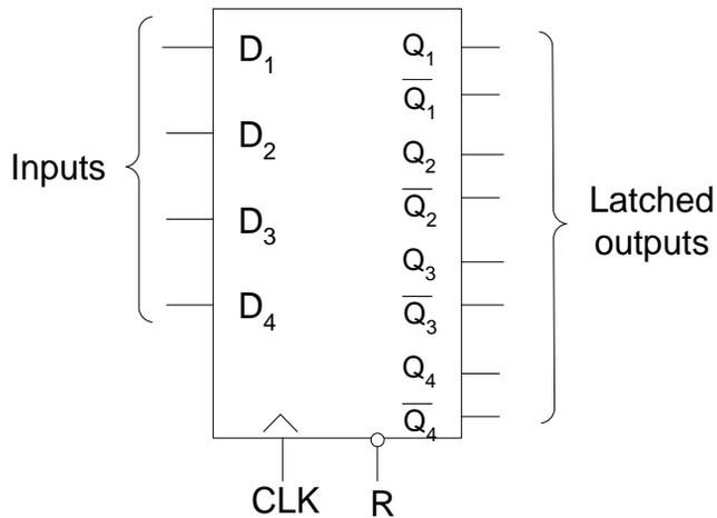
This is quad D register with true (Q) and complemented ( $\bar{Q}$ ) outputs.
