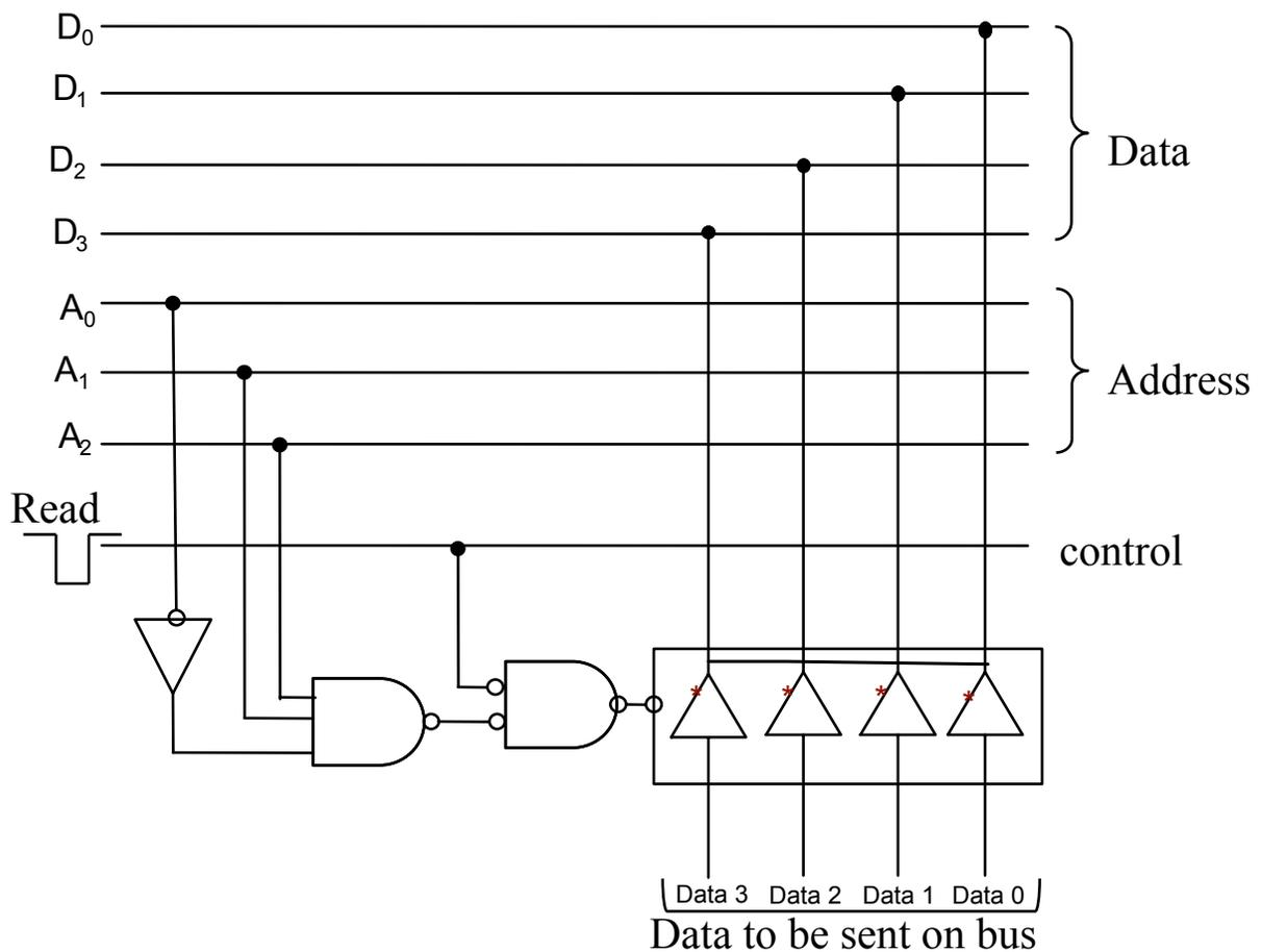
In the above example the device “looks” at address lines  $A_0 - A_2$  and asserts data onto data bus  $D_0 - D_3$  when it sees its particular address line and it sees a READ pulse. However, there must be external logic to control 3 - state devices with the same output lines.
