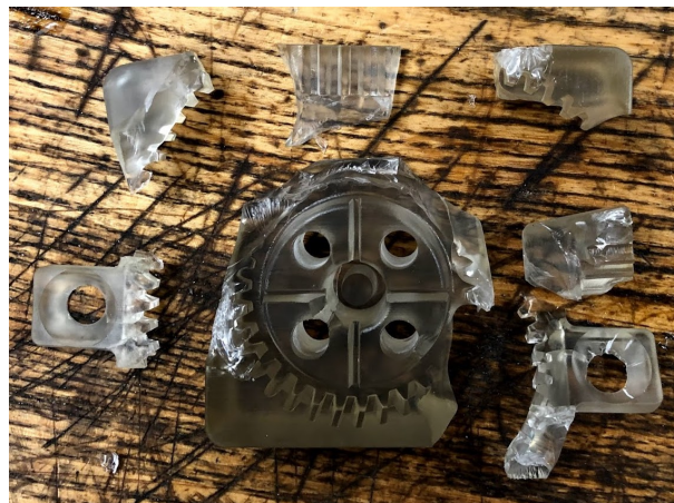
Figure 4.8: Fractured pieces of the High Temperature resin SLA mold (60 min cure).
