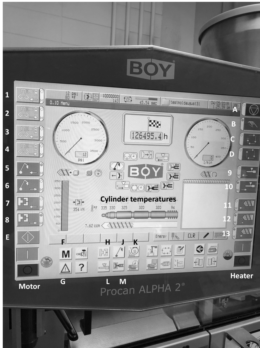
Figure 2.4: Labeled photo of BOY 35E user interface.
