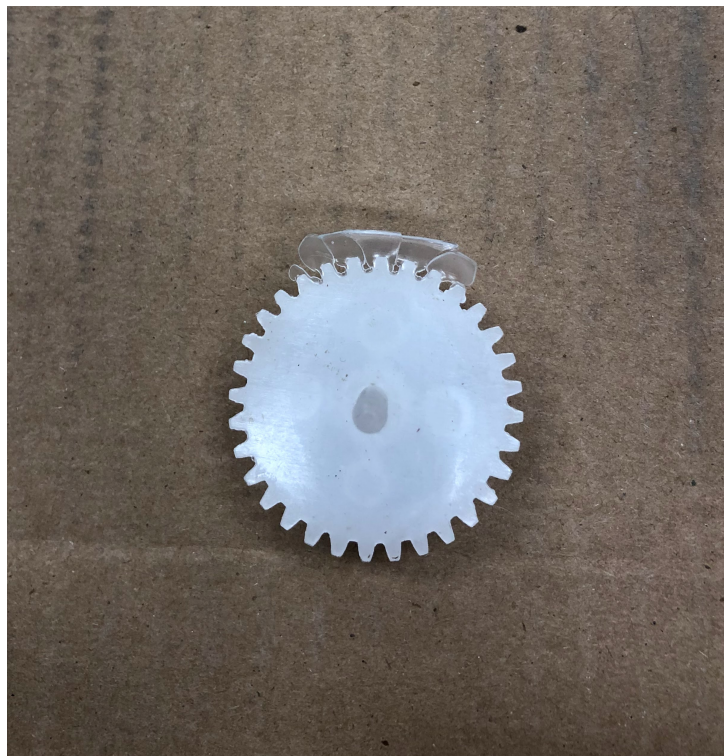
Figure 5.2: Injection molded gear with flash.
