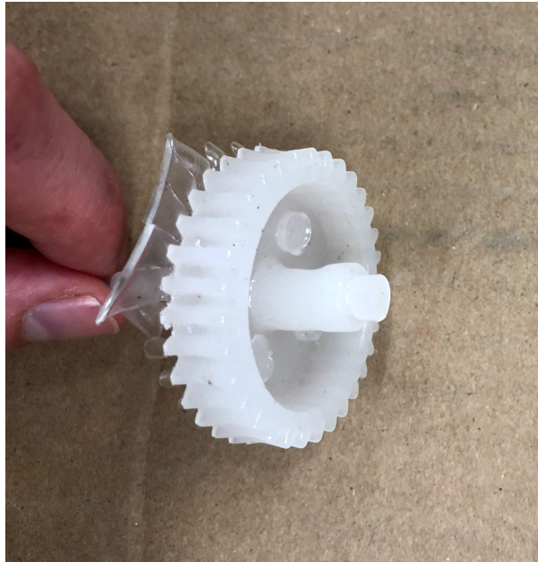
Figure 4.5: An injection molded gear with flash and a sink mark on the gear hub.
