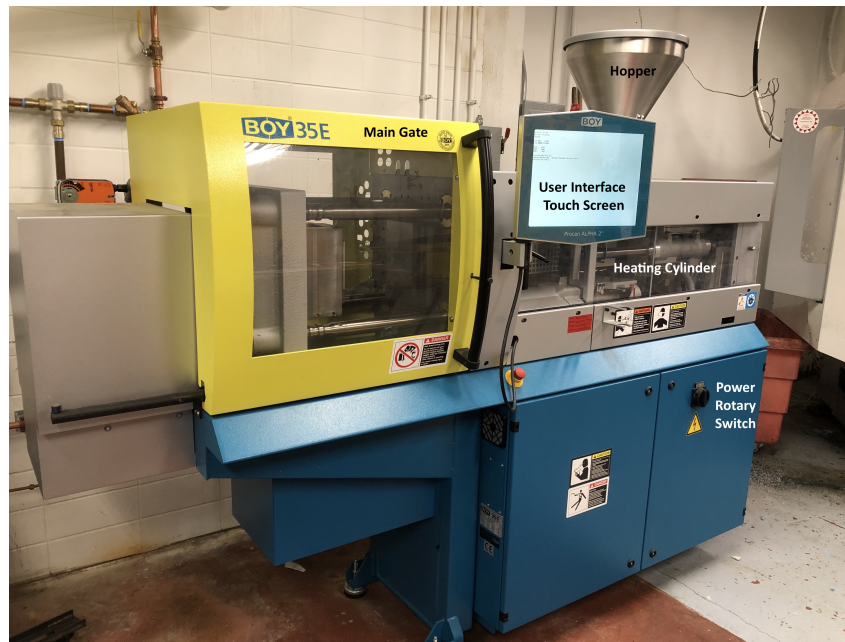
Figure 2.1: Labeled photo of Princeton's BOY 35E Procan Alpha.
