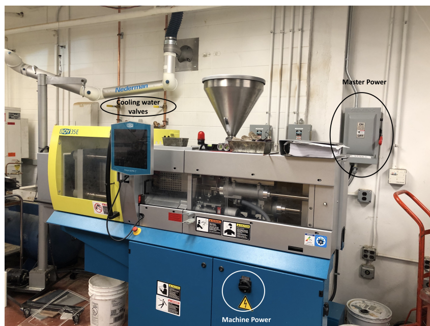
Figure 1.1: Photo of injection molding machine with power and water cooling valves labeled.
