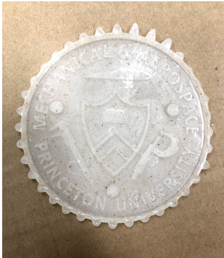
Figure 5.1: Injection molded coaster which has burn marks, air bubbles and is underfilled.
