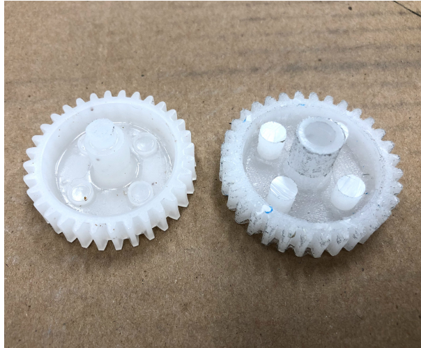
Figure 4.4: Comparison of a gear produced using an FDM mold (right) and a gear produced using an SLA mold (left).
