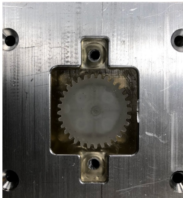
Figure 4.9: Nearly imperceptible cracks in the SLA mold (30 min cure).
