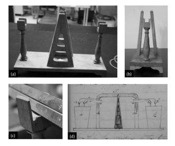
Fig. 8. Stand that supports the rocking armature: (a) front view; (b) side view; (c) wooden support for holding magnet; and (d) 1842 sketch from a student notebook showing the A frame.
