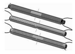
Fig. 4. Illustration of one of the two possible windings of wires in the Princeton motor armature showing iron core, whiskers, and coil attachments. At the top is the outer winding, in middle is the inner winding, and at the bottom are both windings.
