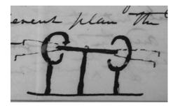
Fig. 11. Henry sketch of motor with C-shaped permanent magnets from his letter to Green in 1834 (Ref. 6).
