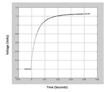
Fig. 5. Voltage versus time across R in the series LR circuit showing an exponential rise; a fit to this curve is used to determine a value for L.
