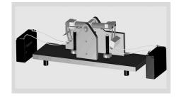
Fig. 14. Replica of the 1831 motor using brush-type contacts instead of mercury-filled cups constructed to test motor dynamics.
