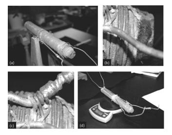
Fig. 3. Closeups of the Princeton motor armature: (a) appearance in its normal operating position on stand; (b) end of iron core showing cloth liner; (c) wire connection of one coil to a whisker; and (d) armature being weighed on a laboratory scale.
