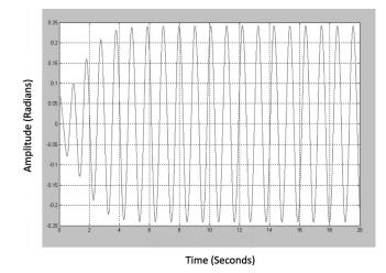
Fig. 15. Graph of armature angle versus time according to the improved motor model, showing the ability to speed up and increase its amplitude.
