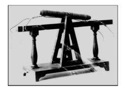
Fig. 2. Photograph of the Princeton motor, a modification of the 1831 motor, as displayed to the public since 1884.
