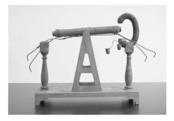
Fig. 10. Princeton motor with the C-shaped electromagnet. Note the proximity of the poles of the armature and the poles of the electromagnet. Note also the wide range of angles possible if the armature was rocking.
