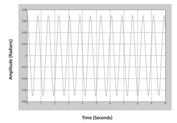
Fig. 12. Graph of armature angle versus time showing the oscillations according to a simple mechanical model of the motor.
