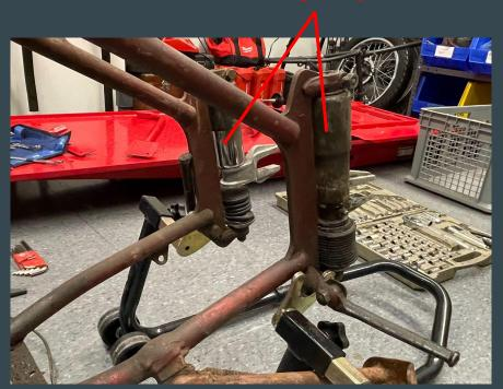
On each side, the rear suspension has two springs, a main and a rebound one below—so four in total. Compressing and extending the springs allows the motorcycle to retain energy, like with the front forks.
