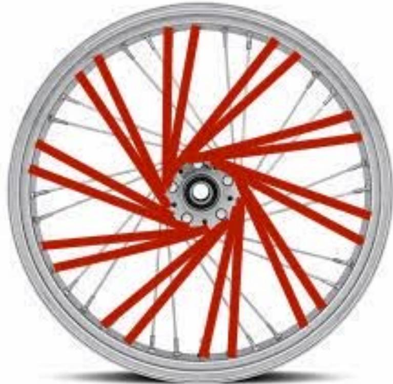
Forward leaning 20 spokes provide tensile reaction
