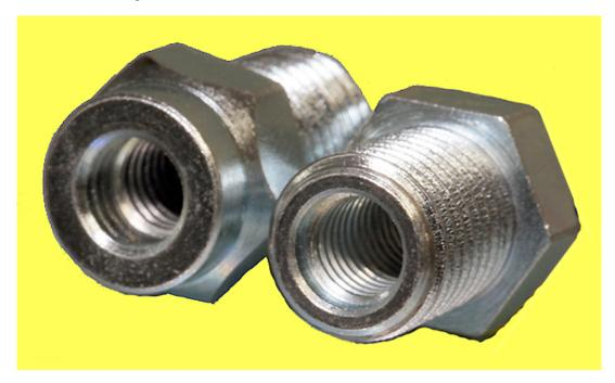
This illustrates that the internal threads of the main/needle jet holder are counter bored.
