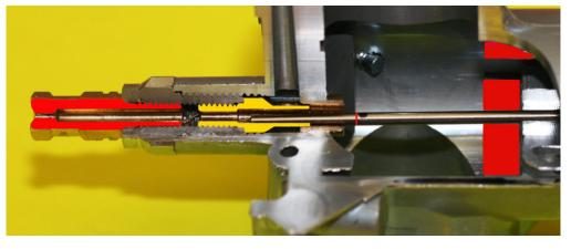
**Slide at Full Throttle:** At full throttle the tip of the needle is clear of the Needle Jet orifice. Depending upon which needle groove the clip is in the Needle stops having any effect around 3/4 throttle.
