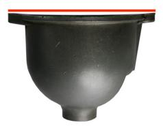
• A warped float bowl from over tightening the float\_bowl screws. The fuel supply passage for the pilot jet passes fuel from the float bowl to the main carburetor body through the float bowl gasket. If the bowl is warped the gasket will leak air into the pilot fuel passage. Fuel will not be delivered to the pilot circuit. If the bowl is warped it must be flattened, or replaced.
