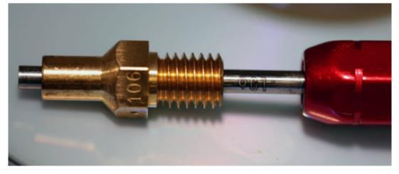
Checking new needle jets. Pictured is a minus .106" plug gauge. It measures .1058" and should be a slip fit in the needle jet orifice. A .106" plug gauge would be a light press fit and a plus plug gauge (.1062") would be a press fit. The small hole on the side of the hex is .035".
