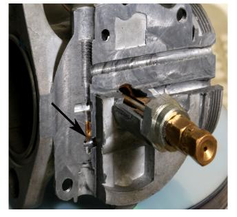
The pilot jet is pressed into the body. The arrow is pointing to the location of the .016" pilot jet's orifice. You can see the two air passages. One is in the center and leads to the needle jet. The other is at the top and leads to the pilot air screw and the fuel supplied by the pilot jet. The two transfer orifices, primary and secondary, are located the slot between the pilot jet and the tip of the pilot air screw.
