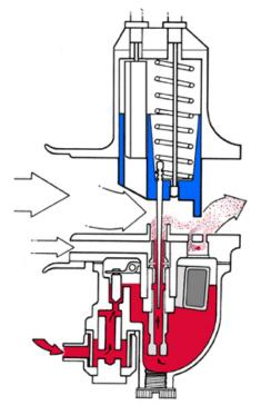
As the Slide is lifted: The Secondary transfer port reverses flow and is now drawing fuel from the mixing chamber adding to what is coming out of the main carburetor's spray tube. It sort of acts like an accelerator pump in an automobile carburetor.
