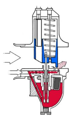
The slide is in the idle position. The secondary transfer port under the back edge of the slide is taking in air into the small mixing chamber just under the two transfer ports. The fuel/air mixture that supports idle is ONLY coming out the small primary port just behind the back edge of the slide.
