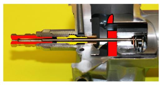
**Slide at 1/2 Throttle:** At 1/2 throttle the fuel metering is clearly being done by the needle's taper.
