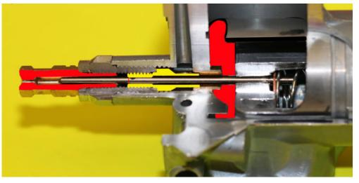
**Slide Closed (idle):** (Red line on needle beginning of taper. From the slide closed up to approx. 1/3rd throttle the fuel metering is controlled by the i.d. of the needle jet and the straight portion of the needle.
