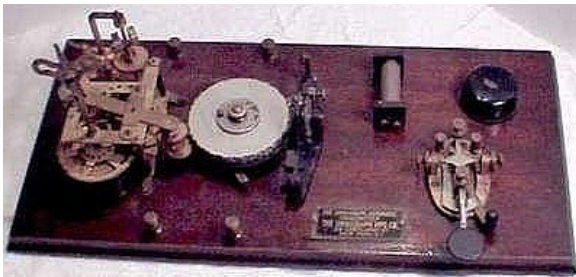
Fig. 13: Omnigraph No. 2 Junior with integral buzzer, key, and provision for use with earphones.
