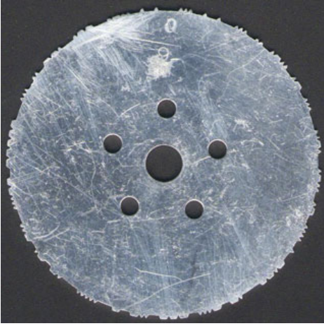
Fig. 4: A typical disc used on a single disc Omnigraph instrument. A single central spindle hole holds the disc onto the rotating platter. This particular disc is marked "6". Transcription of the American Morse reads: "HR STMH FM NEW YORK 21 TO ADH. YES SIG LH"
