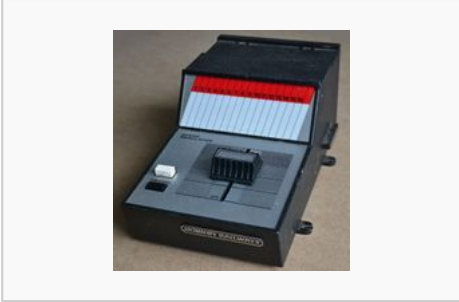
R945 Slave Unit, which attached to the Master unit. Note the 16 "slots" on the label for making notes of which engine was on that channel.
