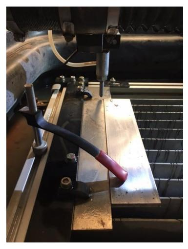
12) IMPORTANT!! Move the axis to the exact start position and set part zero.
