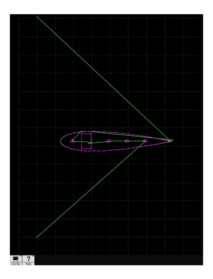
This model looks OK but many times the cut needs to be changed. Also the lead in and out are very long. These can be shortened by using divide, Select, Delete.
