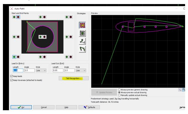
Pick Go. The purple as stated are cut lines and the green are rapid movement with no cutting yellow are the lead ins, they are cutting.
