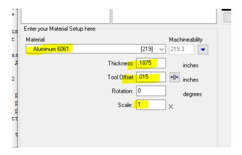
Also: Make sure that your Tool Offset is .015" if you are cutting along the sketch and leaving the line (preferred). If you want to cut the sketch on the line, fill in 0.0". Using 0.0" will cut on the line creating a cut of .015" on each side of the line due to the nozzle cutting width.
