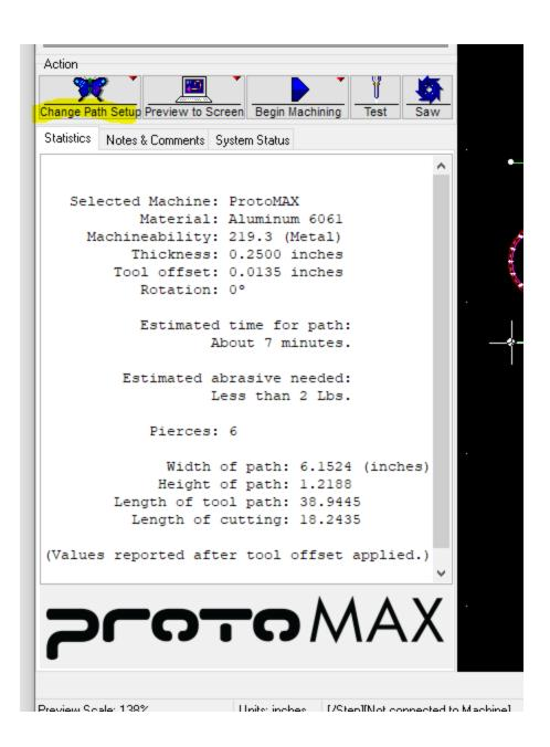
5) Fill in the proper material and thickness.
