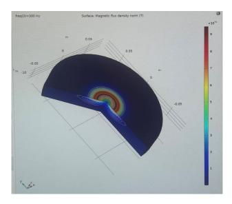
The above animation demonstrates the decreasing of the magnetic field over the time interval of three seconds with a constant frequency of 300 Hz with a copper coil simulating the inductive copper wire.  $\parallel$
