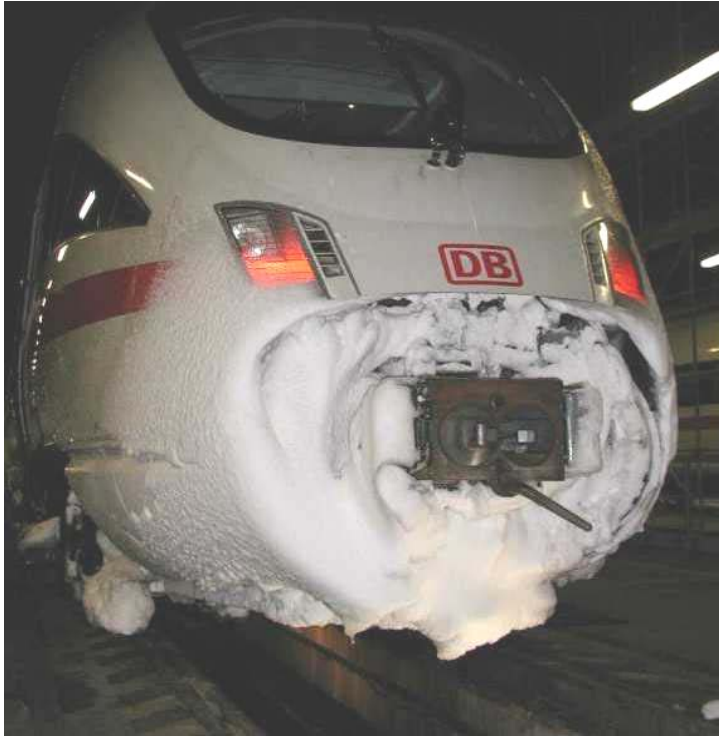
Figure 20. A German class VT 605 with snow packed in the coupler pocket. 16
