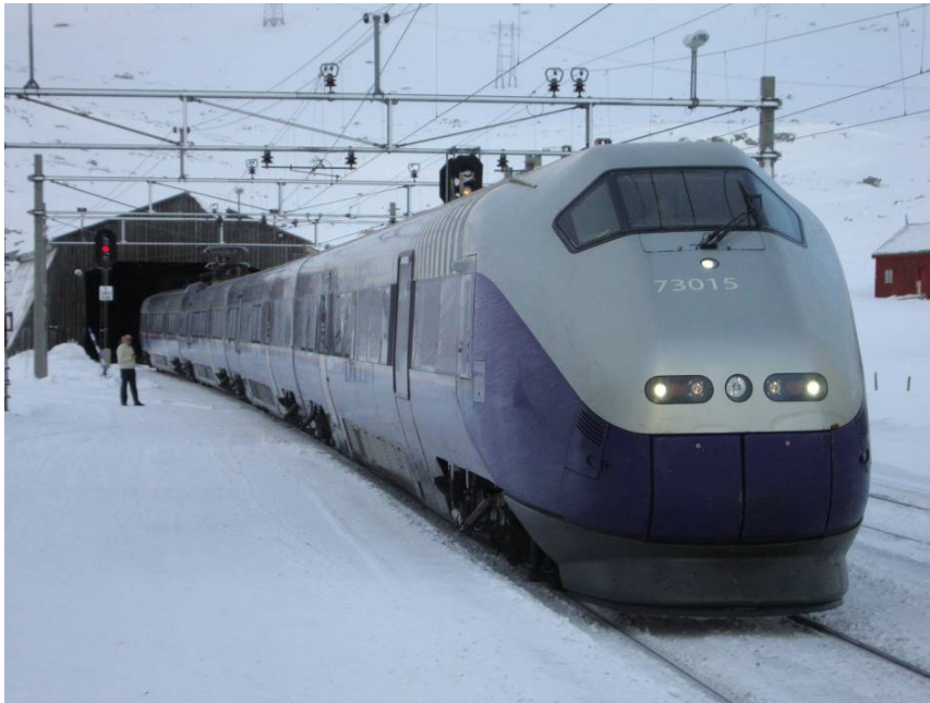
Figure 34. A Class 73 approaches the Norwegian station Finse on Bergensbanen in January 2010. Notice the lack of snow and ice on the train.
