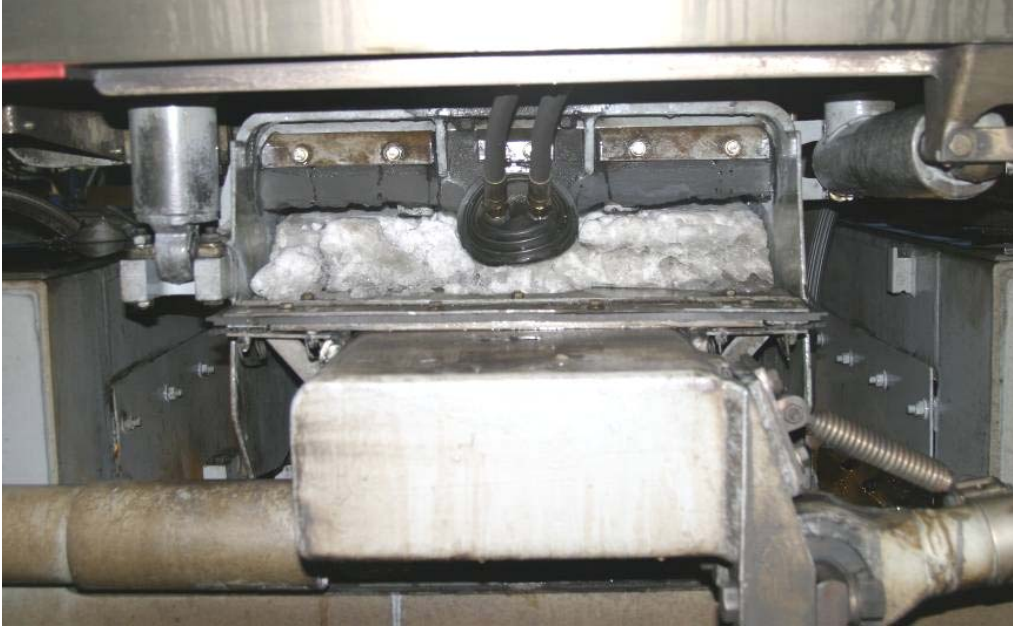
Figure 16. A rubber seal is mounted to prevent the snow to come further into the X2 tilt mechanism.
