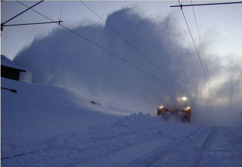
Figure 50. Demonstration of a 1440 hp rotary Beilhack snow thrower at Finse in January 2010 on Bergensbanen.
