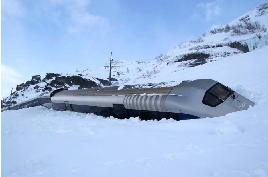
Figure 39. The couplings did not break and the train unit came to a halt in one piece with just the two first cars derailed. 28
