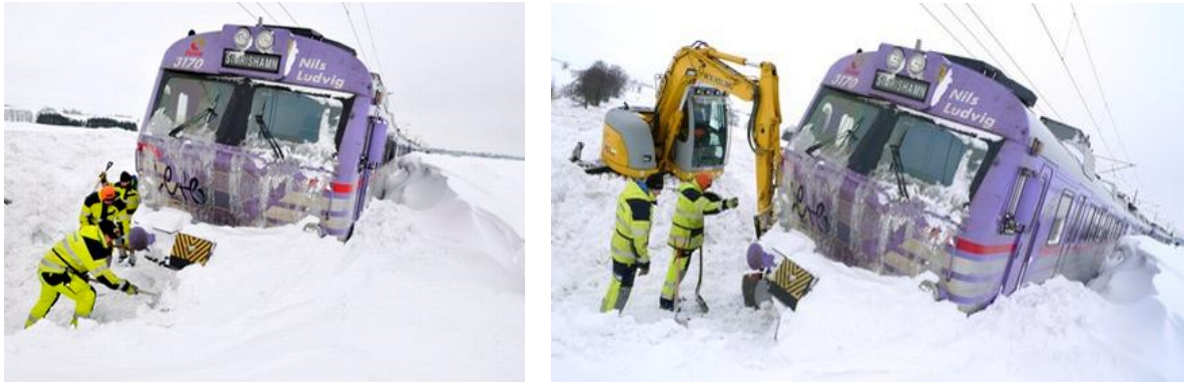
Figure 41. With help from the army the passengers were evacuated from this EMU Class X11 that got stuck between Tomelilla and Simrishamn in the far south of Sweden 32 . Class X11 is a two car unit with 1280 kW and a total mass of 100 tonnes.
