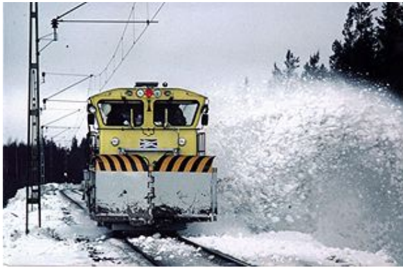
Figure 42. A Swedish (Bo)' (Bo)' Class DLL (ex Class Tb) clears the trackside snow on an electrified line 33 .
