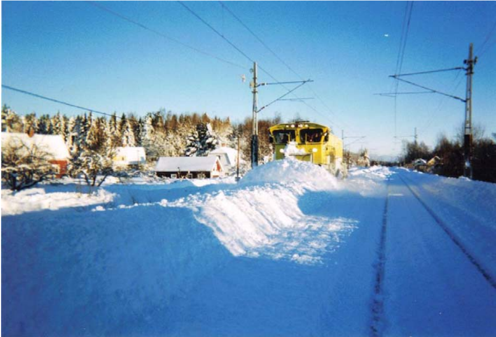
Figure 69. To keep main lines open big snow throwers or ploughing locomotives are necessary. The photo shows a 1235 kW diesel locomotive (ex class Tb) clearing the second track. The main track has already been cleared on this location close to Gävle some 200 km north of Stockholm. 57
