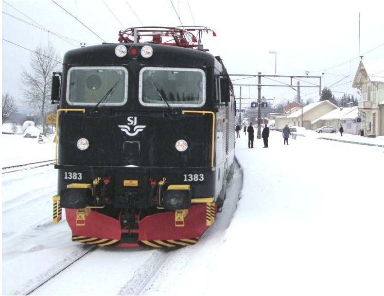
Figure 24. A Swedish Rc locomotive with a standard snow plough heading a Stockholm-Oslo train. The tip is cut off. This is to give a free area for the person doing the coupling and decoupling. It has also the effect that the rear plough does not collect so much snow on the back side as there is a wind stream backwards through the opening.
