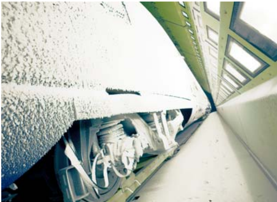
Figure 35. Ongoing winter tests with a deep frozen Siemens Velaro train for Russia in Vienna climatic chamber. 25
