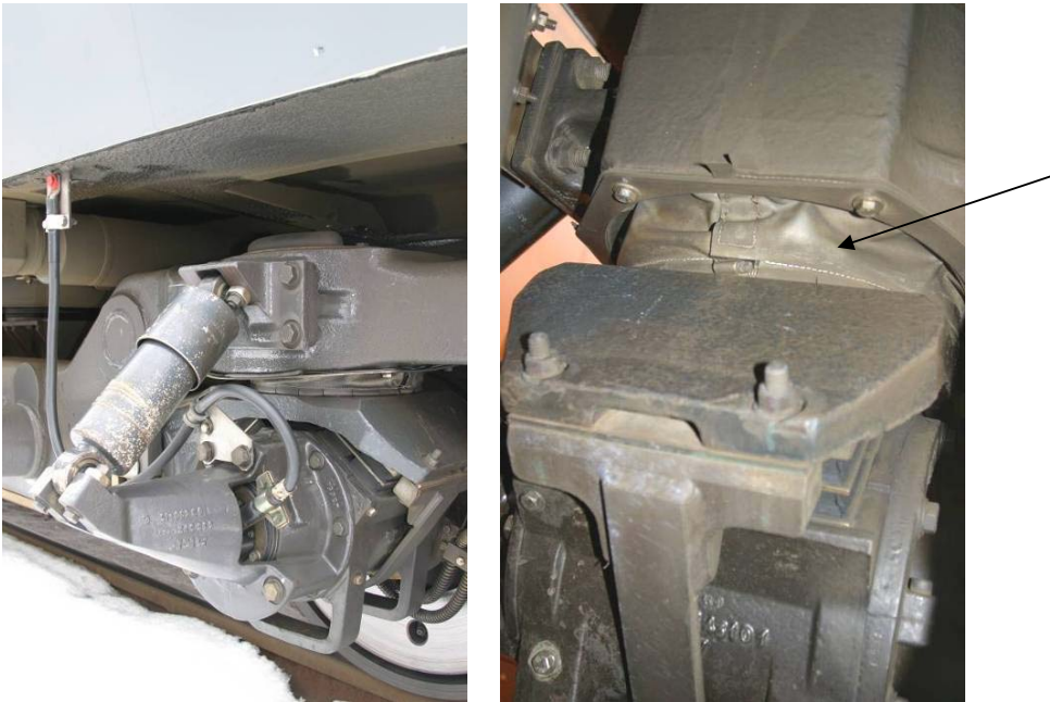
Figure 15. Snow covers/bellows around the primary suspension of the Norwegian BM71 seen from two perspectives.
