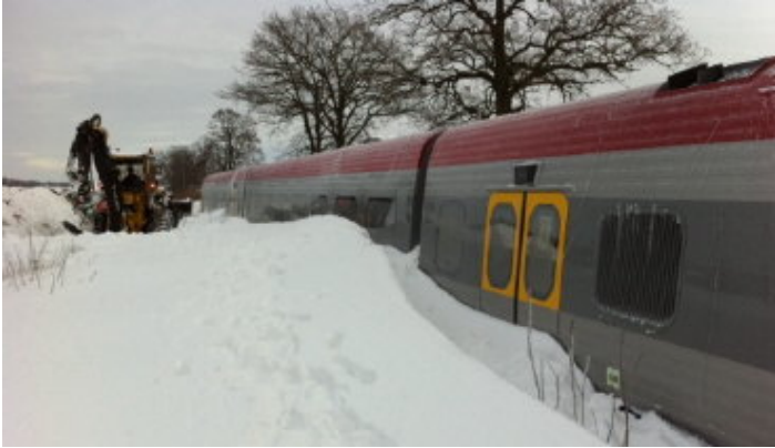
Figure 22. A Swedish DMU Class Y2 stuck in the snow on the Linköping – Kalmar line although the train has got four diesel engines of totally 1240 kW. 18
