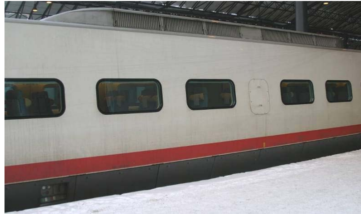
Figure 29. Above: High positioned air intakes on the Finnish Sm3.
