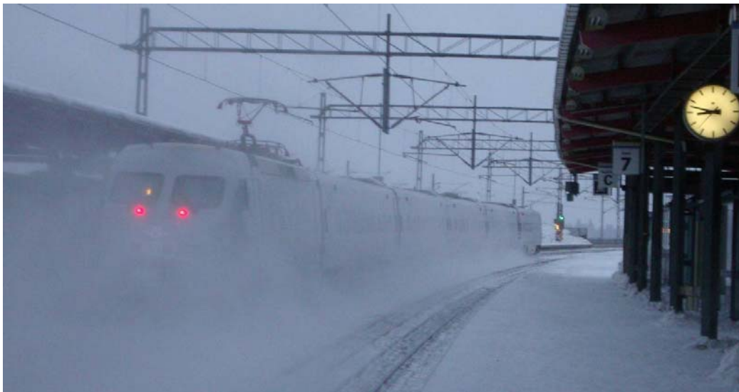
Figure 71 and front figure. Snowsmoke around passing X2 trainset in Södertälje south of Stockholm in January 2010. Notice the intense snow smoke at the bogie level.
