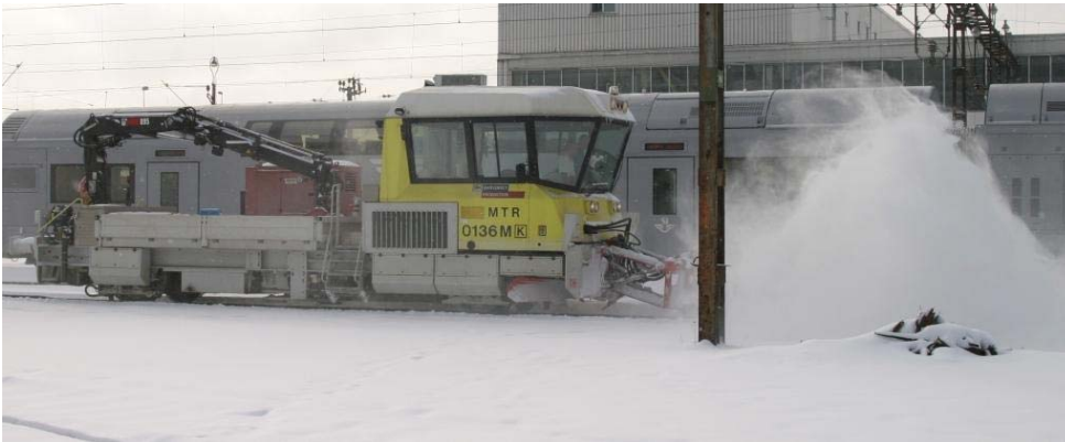
Figure 70. In Swedish yards a two-axle service vehicle often is used for snow clearing, usually with a rotating brush at the front. It is an effective way to clear switches in the beginning of the winter season. However when there is a lot of snow and high snowdrifts, the effectiveness goes down.
