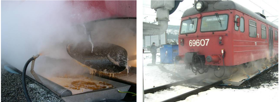
Figure 32. De-icing with propylene glycol in Drammen, Norway. 23
