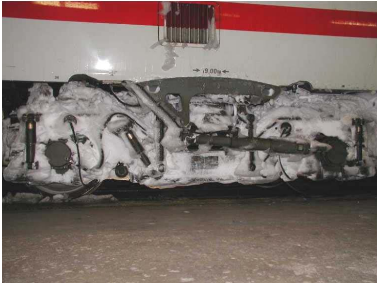
Figure 3. Snow packing in a German bogie VT 605. 4
