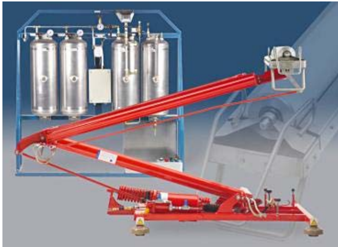
Figure 63. Dummy pantograph for putting glycerol on the contact wire to reduce the arcing 52 .
