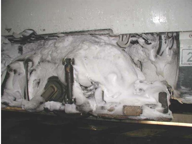
Figure 10. Snow and ice gatherings in a German VT 605-bogie after some time of operation. 9
