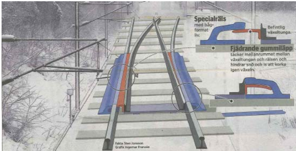
Figure 56. The proposed technical solution with a covering flexible lip that is hidden under the rail head when the switch tongue is closed. 47
