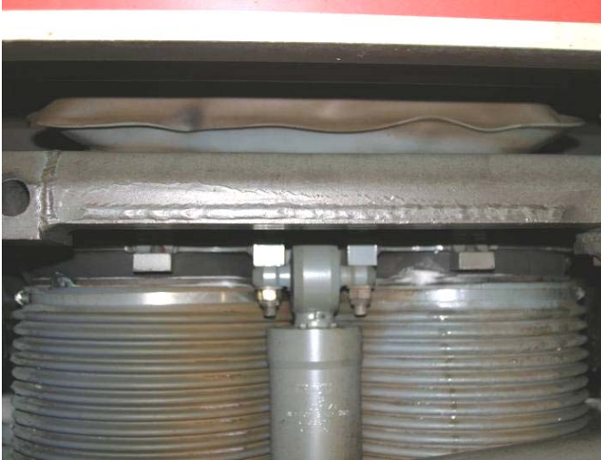
Figure 14. Snow covers both for the secondary coil springs and for closing the gap between the carbody and the bogie frame at the Finnish Sm3.
