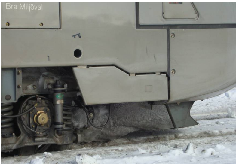
Figure 25. A Swedish Class X40, where the area between the rear bogie and the plough is filled with snow. It can also be seen that a plough mounted so far in under the carbody is more an obstacle deflector than a snow plough.
