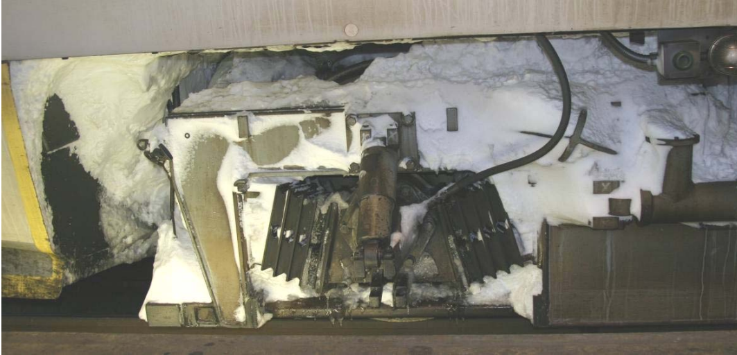
Figure 17. Snow packing in a Class X2 bogie.
