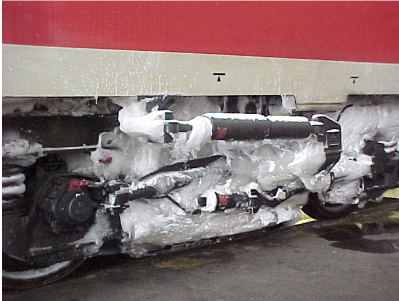
Figure 2. An example of a bogie with adhering ice, a German class VT 612. 2
