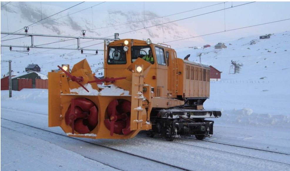
Figure 51. The Beilhack machinery can be turned for operation in both directions.
