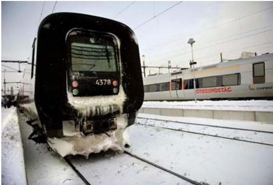
Figure 21. An Öresund train EMU Class X31 for the operation in southern Sweden and in eastern Denmark. The plough may function as an obstacle deflector but as a snow plough it looks like a poor design that does not manage to throw the snow to the side. The equipment behind it, such as the primary dampers seen to the left, is not protected. 17
