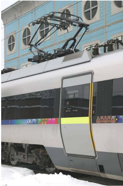
Figure 29. Above: High positioned air intakes on the Finnish Sm3.
