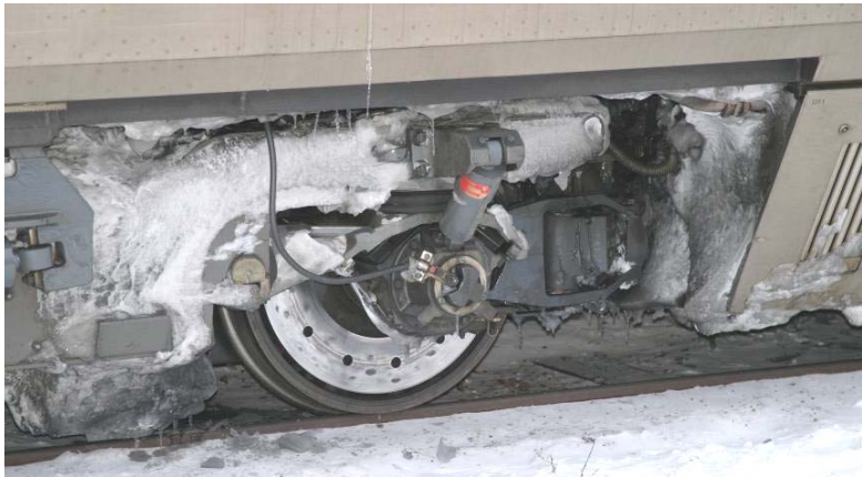
Figure 9. A Swedish Class X2 bogie with snow and ice gatherings, in the beginning of the ice build-up.
