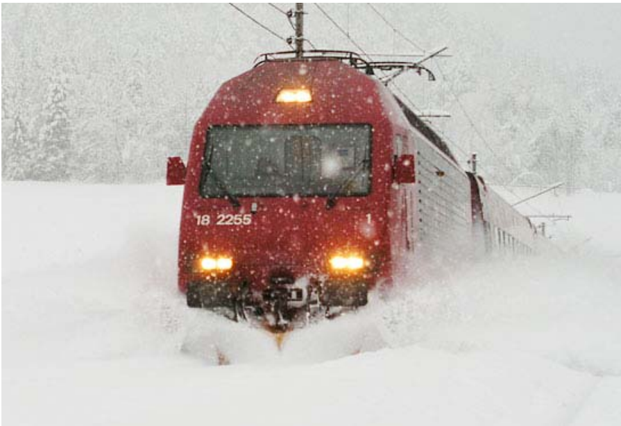
Figure 23. A Norwegian E18 with a passenger train on a not cleared line section. The effect of the angled front plough can be seen as snow smoke thrown to both sides of the locomotive. 19
