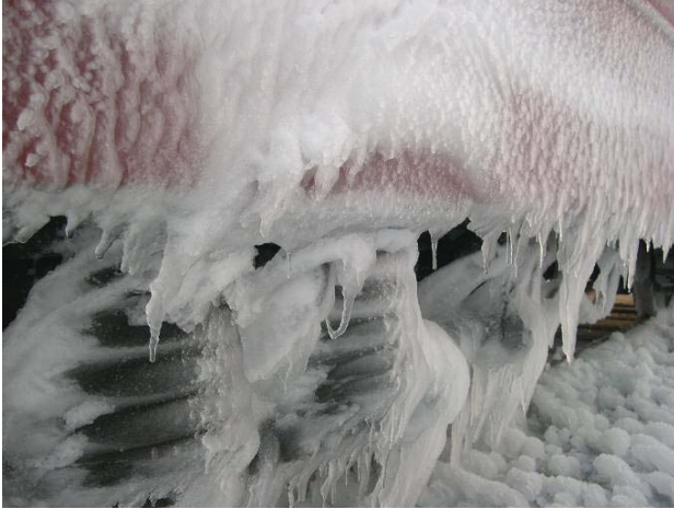
Figure 13. Bogie and carbody covered with ice. 11
