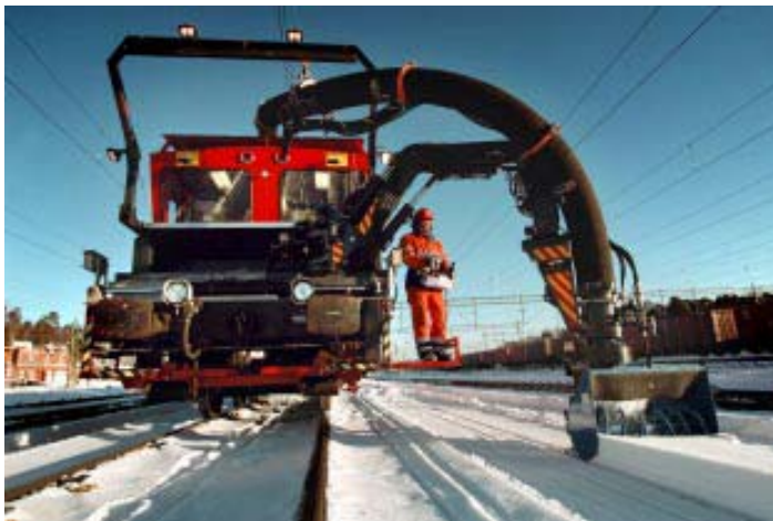
Figure 49. Equipment that sucks the snow in and at the same time melts it with warm water. The water is then sucked further to a container before it is emptied as surface water. The operator can manoeuvre the equipment from a platform on the side of the vehicle for better visibility 42 .
