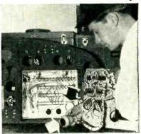
Mid Continent Airline mechanic, S. M. Fabac, holding a Cannon Electric Type "K" Plug about to be installed in the instrument pane of an MCA airliner. Upper black arrow points to K-32S Receptacle. "Major timesavers", say Mid-Continent Airlines of Cannon Plugs.
