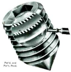
The Knurling of this "Unbrako" Socket Set Screw, as shown "swages the threads", so that it becomes a most excellent "Self-Locker"... for use with the 5 standard points that do not lend themselves to knurling. This "Unbrako" Socket Set Screw positively will not shake loose, regardless of the most chattering vibration. Sizes available from #4 to 1½" diameter, and in a full range of lengths. Ask for your copy of the "Unbrako" Catalog... it is useful and informative.
