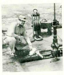
Well attachment ready for firing. Sound traveling down is partially reflected by obstructions and surface of oil
