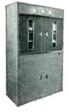
The Western Electric 33C Antenna Control Unit includes a branching circuit and two phase shifters, and permits adjustment of the current ratio and phase relation between the element currents of two towers. This unit handles up to 10 km.
