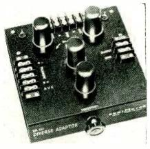
of two antennas for receiving the desired signal on as little as 0.05 volt of avc. It operates on 200 to 300 volts at 15 ma and filament supply of 6.3 volts a-c at 1.5 amperes.
