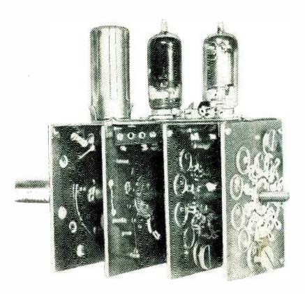
Franklin rotary-switch assembly with die-stamped ransmission lines
