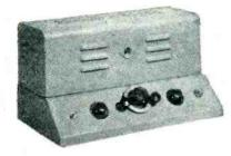
HS-5 alarm detects intrusion by change in antenna capacitance upon approach of a person. It also detects fire by means of a heat detector that operates at about 160 F. Slow capacitance changes owing to changing meteorological conditions will not affect the device.
