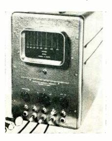
tions in these materials. Using ultrasonic frequencies, the device operates on the basis of thickness vibrations, and gives a cathode-ray presentation of its findings.
