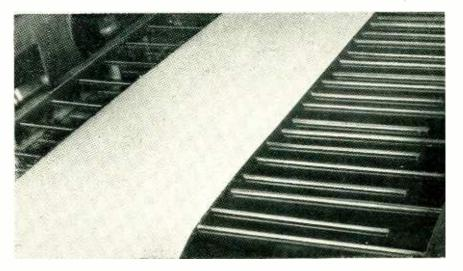
Solvent, used to flow film onto a cellulose backing, is preheated before being removed in an oven. Using the electronic preheater increased productivity of the plant 40 percent
