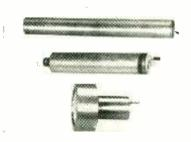
window, thin-wall, and all-metal cosmic ray counters illustrated are completely described in Bulletin 10.
