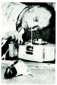
Dr. Gengerelli adjusts transmitter that sends impulses to tiny crystal rectifier placed under skin covering rat's skull. Note antenna wire projecting above rat
