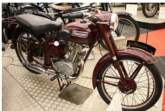
Triumph Terrier T15 150 cc with plunger rear suspension and contact breaker points behind cylinder
