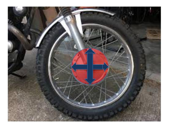
**HUB**—Tension member that supports the spokes. Also connects the wheel assembly to the motorcycle
