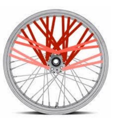
Top 20 spokes provide tensile reaction. Why don't the bottom spokes provide support?
