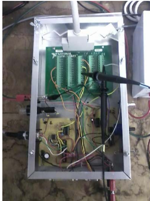
Figure 35: DAQ system. National Instruments Analogue/Digital IO card. Custom built circuit boards: Low pass filter, Digital to Analogue converter for RPM signal, frequency to voltage converter.
