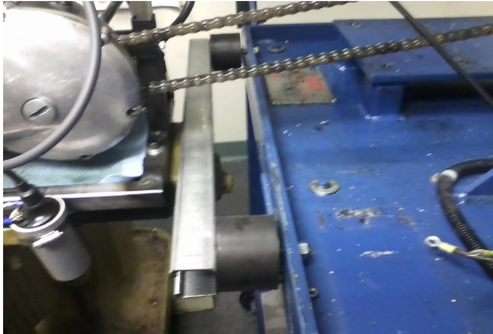
Figure 16: Close up of engine standoff and shock mounts
