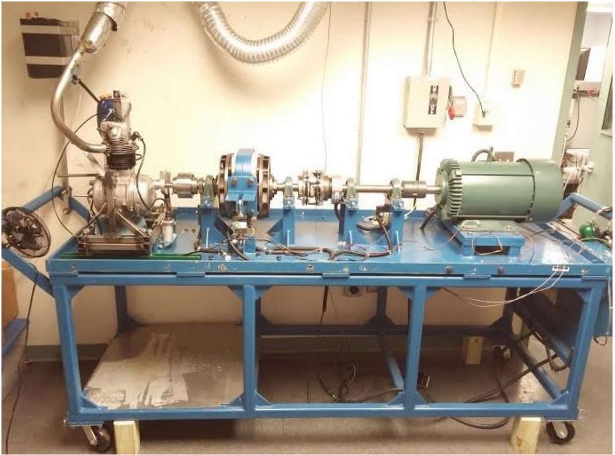
Figure 4: Engine Dynamometer setup with the Triumph motorcycle engine, stands coupled
