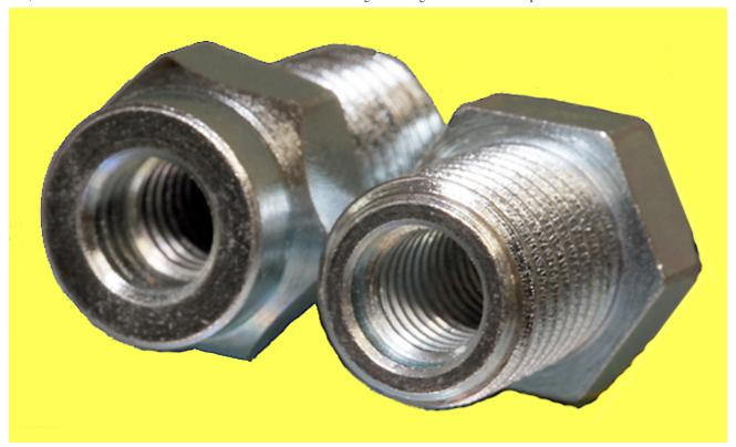
This illustrates that the internal threads of the main/needle jet holder are counter bored.
