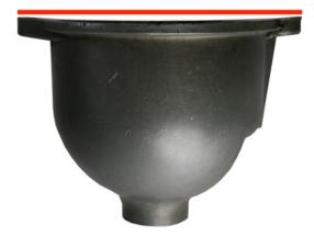
• A warped float bowl from over tightening the float\_bowl screws. The fuel supply passage for the pilot jet passes fuel from the float bowl to the main carburetor body through the float bowl gasket. If the bowl is warped the gasket will leak air into the pilot fuel passage. Fuel will not be delivered to the pilot circuit. If the bowl is warped it must be flattened, or replaced.
