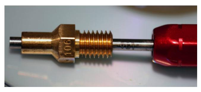
Checking new needle jets. Pictured is a minus .106" plug gauge. It measures .1058" and should be a slip fit in the needle jet orifice. A .106" plug gauge would be a light press fit and a plus plug gauge (.1062") would be a press fit. The small hole on the side of the hex is .035".
