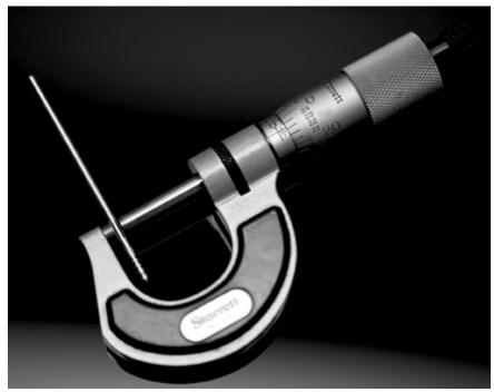
The tapered needle seldom wears to a point where it needs replacing. It can be easily measured on the part that will wear the most, the major diameter. You will find the diameter to be .0985" (2.5mm). The needle grooves are numbered from the top down, with #1 being nearest the top. If the needle is bent it is a candidate to be replaced.
