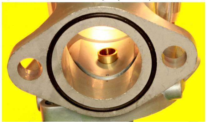
You can clearly see the two pilot transfer holes. The Primary is the smallest at .027", and closest to the reader. The Secondary is larger (.040"), and just behind the groove in the body for the slide. You can also see the brass "Straight Cut" spray tube.
