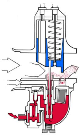
As the Slide is lifted: The Secondary transfer port reverses flow and is now drawing fuel from the mixing chamber adding to what is coming out of the main carburetor's spray tube. It sort of acts like an accelerator pump in an automobile carburetor.
