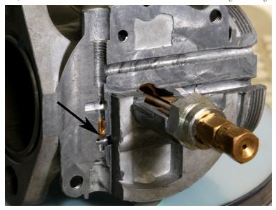
The pilot jet is pressed into the body. The arrow is pointing to the location of the .016" pilot jet's orifice. You can see the two air passages. One is in the center and leads to the needle jet. The other is at the top and leads to the pilot air screw and the fuel supplied by the pilot jet. The two transfer orifices, primary and secondary, are located the slot between the pilot jet and the tip of the pilot air screw.
