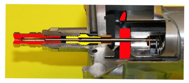
**Slide at 1/4 Throttle:** At 1/4 throttle the needle taper is just beginning to leave the needle jet (as adjusted by the needle clip position).
