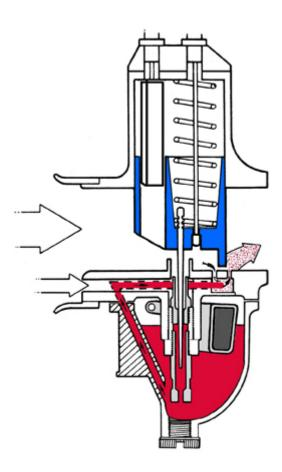
The slide is in the idle position. The secondary transfer port under the back edge of the slide is taking in air into the small mixing chamber just under the two transfer ports. The fuel/air mixture that supports idle is ONLY coming out the small primary port just behind the back edge of the slide.
