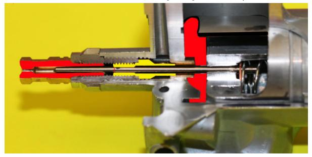
**Slide Closed (idle):** (Red line on needle beginning of taper. From the slide closed up to approx. 1/3rd throttle the fuel metering is controlled by the i.d. of the needle jet and the straight portion of the needle.
