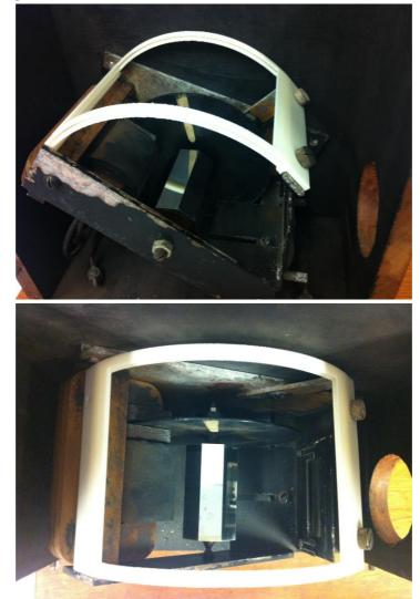
Figure 12 Viewing Box (Including the Screen Holder).
