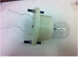
Figure 3 3D-printed Lamp Holder.
