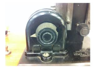
Figure 8 Adjustment Knob of the Potentiometer.
