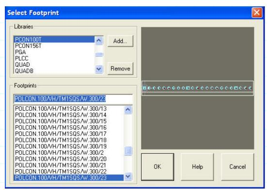
The footprint that comes the closest is the positive lock connector library (PCON100T). We will use the POLCON.100/VH/TM1SQS/W.300/ footprints so that the pins are in the middle of the block and since I need a 12 pin header I will select a 23 pin footprint. I have chosen 23 because my pins are 0.2" apart instead of 0.1" and then take off 1 so the last pin is near the silk screen ([12 x 2] - 1 = 23).
