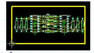
The board we are building only has a top and bottom (no inner layers), so go to Tool -> Layer -> Select from a spreadsheet ...
