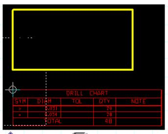
Click on DRC so that it's gray. The Design Rule Checker feature gets in the way at the beginning of the process. The dotted line should disappear.
