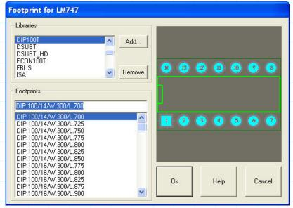
Under footprints, select DIP.100/14/W.300/L.700 which is a DIP Chip with pin that are 0.1" apart, 14 pins, and a component silkscreen (the green box) that is 0.3" X 0.7". Don't worry too much about the silk screen. We buy economy prototyping boards that do not have the silk screen. If we were building full production boards, it would appear as the white writing on the board.
