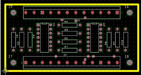
To see the symbols in action hide all layers except "Global Layer", "SST" & "DRD". Hide the layer by selecting it from the pull down menu in the tool bar, and press "-" key. Select the "DRD" layer last so the symbols are on top.
