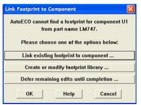
Here's the selection for the LM747. I selected the DIP100T library to give us footprints for Dual In-line Packages whose leads are 0.1" apart, and are Through hole components (versus DIP100B which are surface mount).
