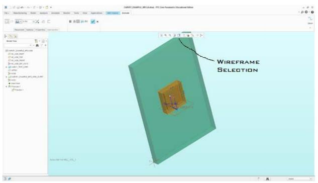
Now we must define a mill volume, which is the only part of the workpiece that the mill will cut.
