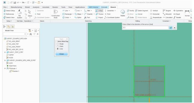
In order to make the most efficient use of material, use the "Offset" tool loop option with an offset of about **0.3** in the sketcher for the extrusion. (If this is too difficult, simply make a rectangle cutout of the material.)
