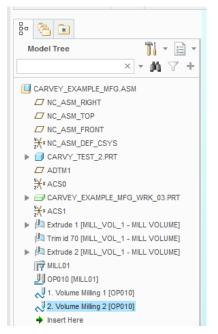
(Depending on which configuration you are using, you will have one or two volume milling entries)
