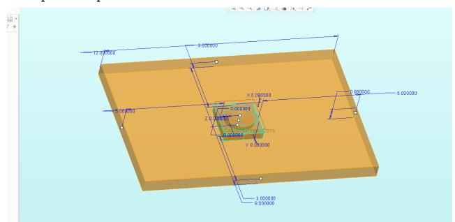
Then, adjust the workpiece dimensions until it matches the dimensions of the stock material you are using by clicking on the blue dimensions and editing them. Make sure to position the part where you want it cut out of the workpiece.
