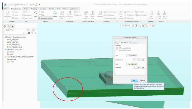
The mill volume will be defined by an extrusion from the face of the workpiece
