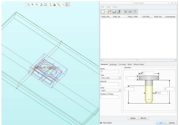
In the above picture the dimensions of a simple ball-end mill have been entered. Hit "Apply" when your tool is set up, then hit "Ok".
