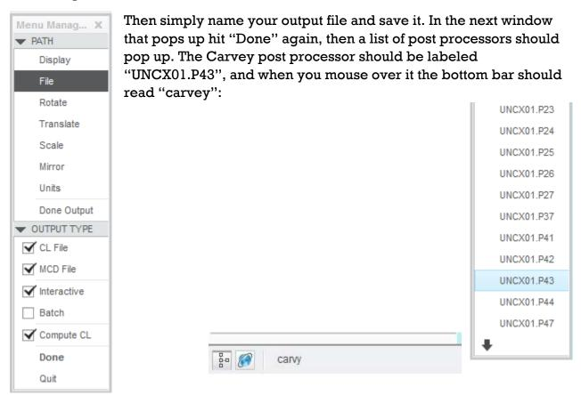
At this point, several dialog boxes will pop up followed by a processing report. Make sure that it doesn't indicate any errors, then you can validate your G-Code by going to the "Play Path" icon in the "Manufacturing" tab and selecting "Material Removal Simulation" from the dropdown menu.
