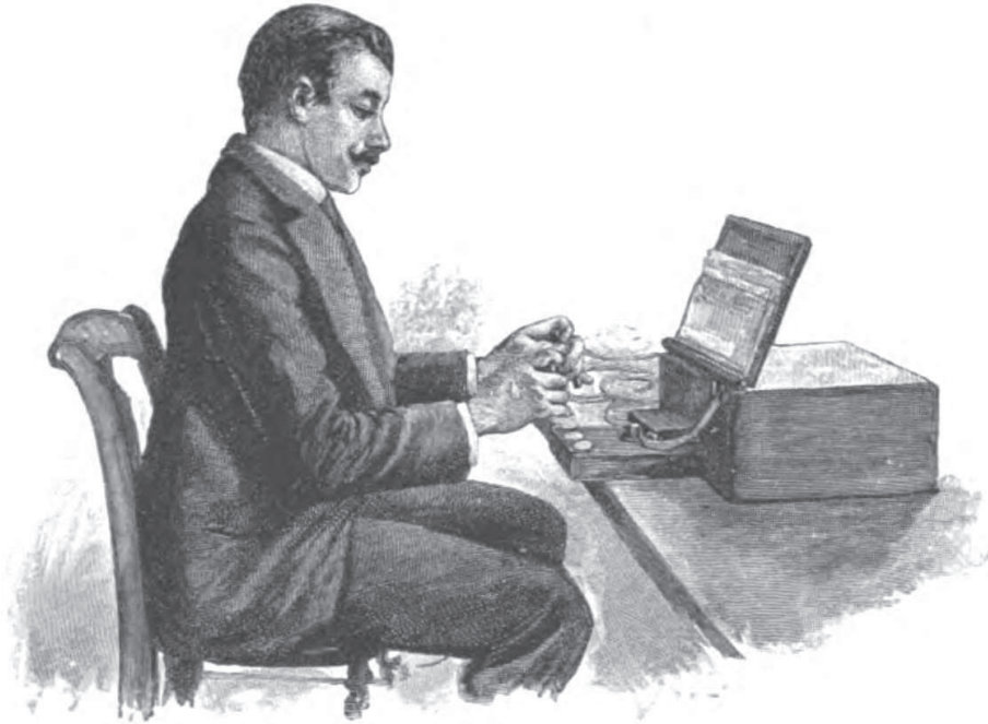
Perforating Messages to be Sent by the Wheatstone System.
