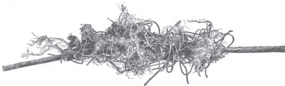
Section of Cable, Chafed and Torn by an Anchor.
