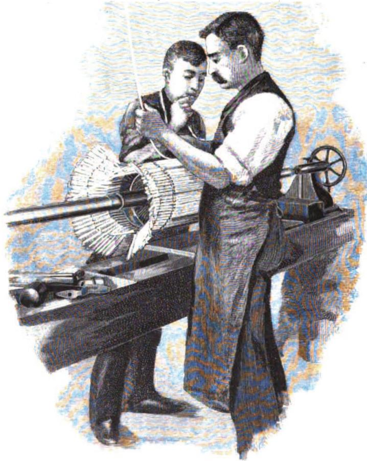
Fig. 7.—Winding an Armature.
