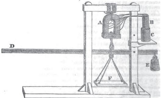
A, the magnet covered with linen, the ends of the wires projecting so as to be soldered to the galvanic element B. C, a cup with dilute acid on a moveable shelf. D, a graduated lever. E, a counterpoise. F, a scale for supporting weights; when a small sliding weight on the lever is not used; a second galvanic element is attached to the appparatus so that the poles of the magnet can be instantly reversed, this is omitted in the figure.
