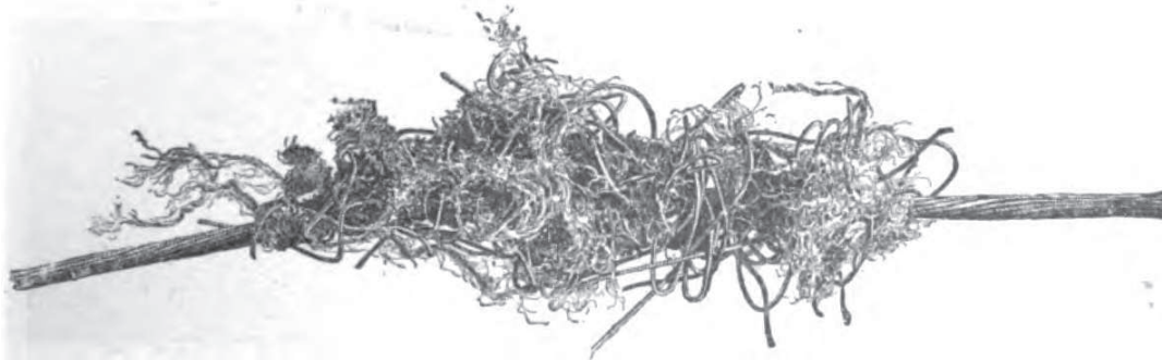
Section of Cable, Chafed and Torn by an Anchor.
