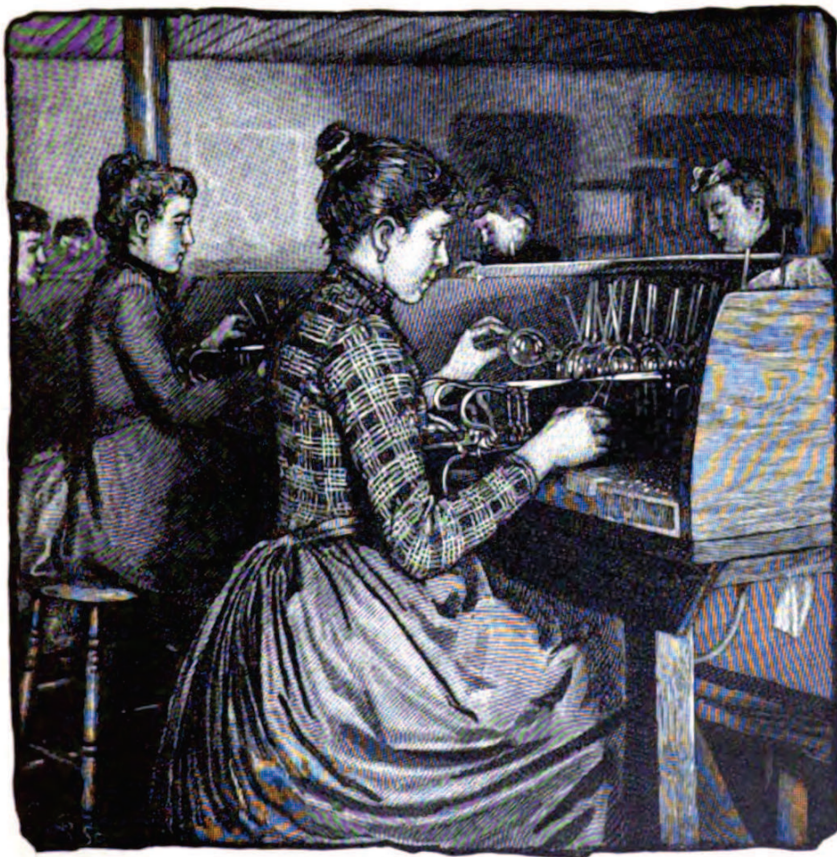
Fig. 20.—Sealing the Glass Socket and Carbon Filament into the Flask of an Incandescent Lamp.
