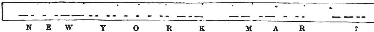
Specimen of Perforated Slip for Sending Message by the Wheatstone; same message as received.
