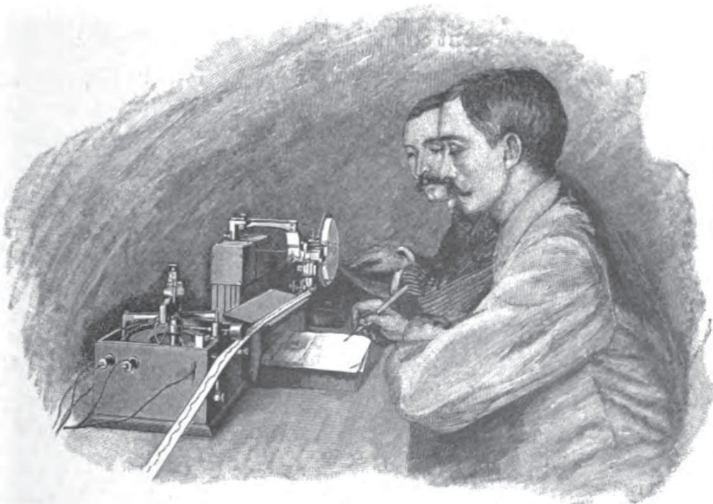
The Siphon Recorder for Receiving Cable Messages—Office of the Commercial Cable Company, New York.
