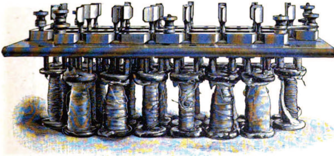
Resistance Coils, removed from box; showing their connections by means of plugs between metallic blocks.
