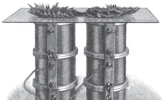
The Magnetic Field, as indicated by iron filings thrown upon a pane of glass resting upon the poles of an electro-magnet.
