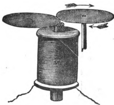
FIG. 121.—Revolution of a "Shaded" Copper Plate held over the Pole of an Alternating Current Electromagnet.
