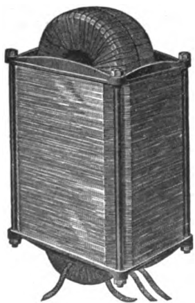
Fig. 25.—Converter or Transformer Used with an Alternating Current.
