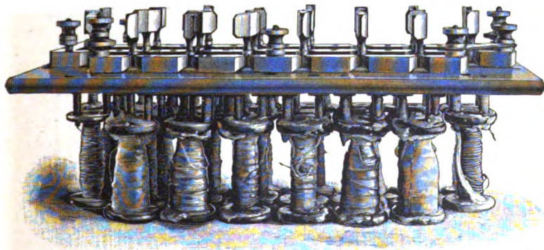
Resistance Coils, removed from box; showing their connections by means of plugs between metallic blocks.
