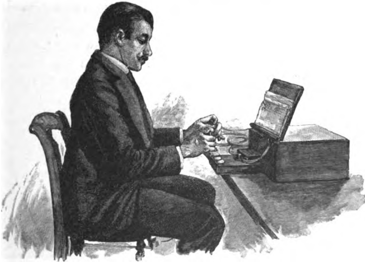
Perforating Messages to be Sent by the Wheatstone System.
