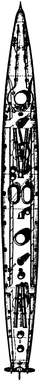
Deck-plan of Yarrow Torpedo-boat, showing discharging tubes mounted on turn-tables.
