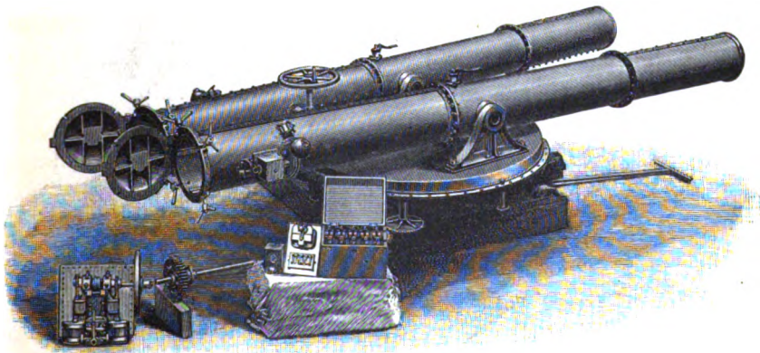
Revolving Deck Tubes for Yarrow Torpedo-boats, showing electrical discharging apparatus.
