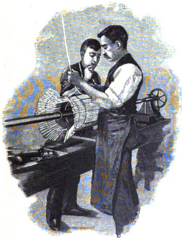
Fig. 7.—Winding an Armature.
