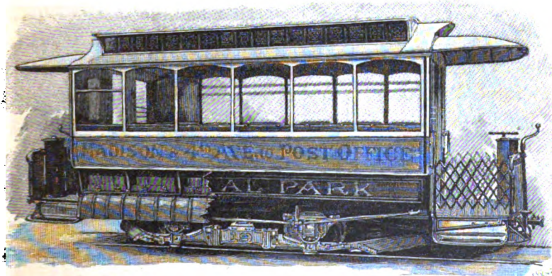
Fig. 9.—The Storage-battery System.—Car of the Julien Electric Traction Company, as run on the Fourth Avenue Road, New York.
