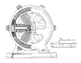
"Dynamo Electric Machine" (end view, partly section, U.S. Patent 284,110)
