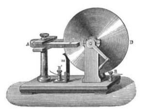
The Faraday disk was the first electric generator. The horseshoeshaped magnet (A) created a magnetic field through the disk (D). When the disk was turned, this induced an electric current radially outward from the center toward the rim. The current flowed out through the sliding spring contact m, through the external circuit, and back into the center of the disk through the axle.
