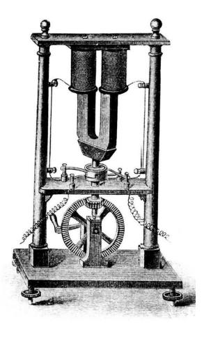
Hippolyte Pixii's dynamo. The commutator is located on the shaft below the spinning magnet.
