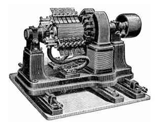
This large belt-driven high-current dynamo produced 310 amperes at 7 volts DC. Available 1917. Dynamos are no longer used due to the size and complexity of the commutator needed for high power applications.
