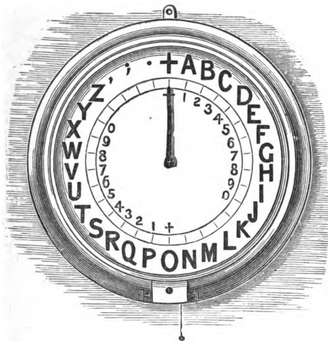
FIG. 70.—Wheatstone's enlarged Dials, such as are used in the engine rooms of Ships of War.
