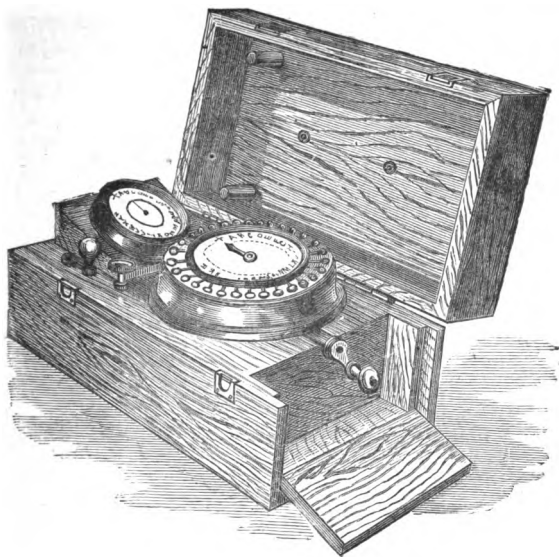
FIG. 60.— Wheatstone's new Magnetic Alphabetic-Dial Telegraph.
