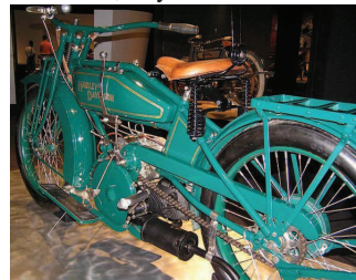
1919 Harley-Davidson Model W Sport Twin. 36 cu in (590 cc), Power: 6 bhp (4.5 kW). Top speed: 50 miles per hour (80 km/h). Memphis exhibition, July 2005.
