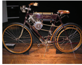
1900 Thomas. 1.8 bhp (1.3 kW), top speed 25 mph (40 km/h). Memphis, July 2005.
