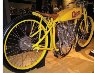
1914 Cyclone. 61 cu in (1,000 cc). Power: 45 bhp (34 kW) @ 5,000 rpm. Top speed: unknown. Memphis exhibition, July 2005.
