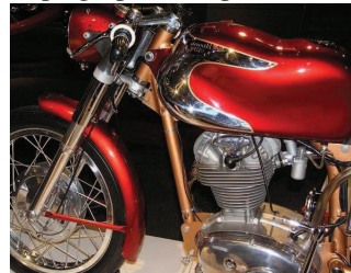
1962 Ducati Elite. 204 cc (12.4 cu in). Power: 17 bhp (13 kW) @ 7,500 rpm. Top speed: 85 mph (137 km/h). Memphis, July 2005.
