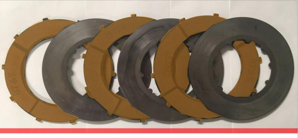
These six objects constitute the innards of the clutch basket: three 'driving plate' alternating with three 'driven plates.'
