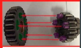
THE EXTERIOR TEETH ON BOTH SIDES OF THE SECOND GEAR FIT INTO THE RECESSED TEETH ON THE ADJACENT SPROCKETS
