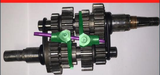
This is what the selector forks look like in place. The rod is attached to the inside of the engine case, ensuring that the forks move along the same, consistent line.
