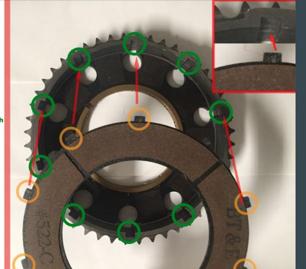
THE TEETH ON THE **INSIDE OF THE DRIVEN PLATE** FIT INTO THE RECESSED **TEETH ON** THE SHOCK ABSORBER, **WHICH IN TURN ROTATES THE TRANSMISION** (ON THE OTHER SIDE OF THE **BOTTOM END)**
