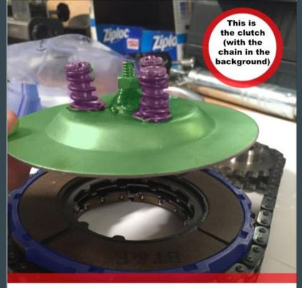
The pressure plate is pressed by three springs so that it pushes together the driving plate and the driven plates, located within the cluch basket, causing them to rotate together.
