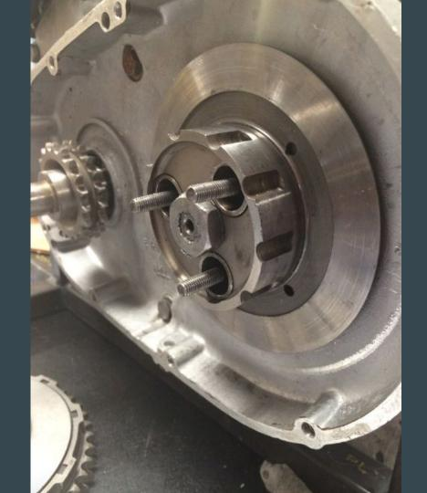
The driving plate (at right) have four sections made of cork (one of which is outlined in purple). This means that when the springs on the pressure plate are in their default position of pressing the driving and driven plates together, the friction created by the cork quadrants on the driving plates forces all siz plates to rotate in unison.
