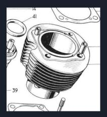
It's important to make sure the cylinder and piston fit perfectly with one another so that the engine is as efficient as possible without seizing up.
