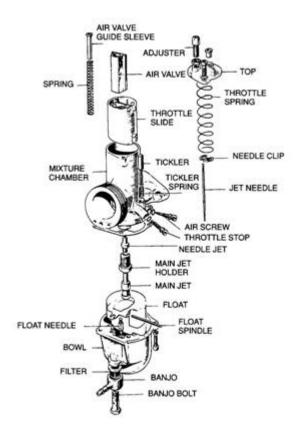
For slow running, set the twistgrip to make the engine run slowly but just faster than at tickover. Then gently screw in the throttle stops to just hold the valves in that position, and return the twistgrip into the shut position, leaving the engine running on the throttle stops. The next thing to do is to set each carburettor to obtain the idling by screwing down the throttle stop screws and adjusting the pilot air screws accordingly.
