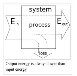
In general, energy conversion efficiency is the ratio between the useful output of a device and the input, in energy terms. For thermal efficiency, the input,  $Q_{in}$ , to the device is heat, or the heat-content of a fuel that is consumed. The desired output is mechanical work,  $W_{out}$ , or heat,  $Q_{out}$ , or possibly both. Because the input heat normally has a real financial cost, a memorable, generic definition of thermal efficiency is<sup>[1]</sup>
