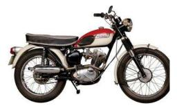
Triumph Tiger Cub Claimed power: 10hp @ 6,000rpm (14.5hp @ 6,500rpm/Sports-Mountain Cub) Top speed: 60/70mph Engine: 199cc air-cooled OHV single
