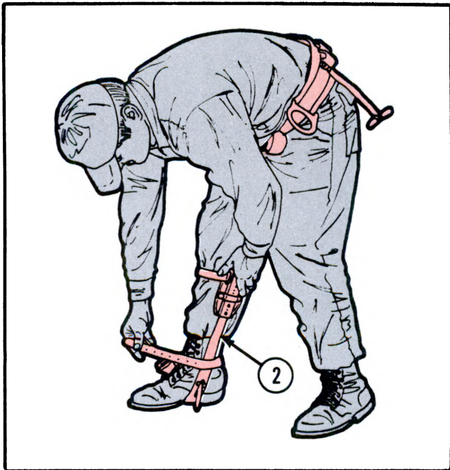
2 Strap the leg irons (2) to the legs and feet.
