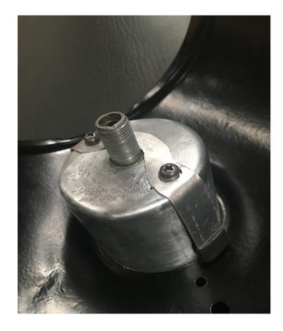
We made a new fitting to keep the speedometer in place, shown above.
