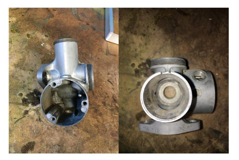
The base of the carburetor was extremely dirty, so we used wire brushes to remove the grit.
