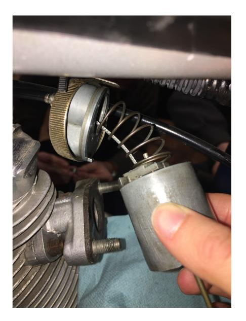
This is how the throttle cable attaches to the carburetor.
