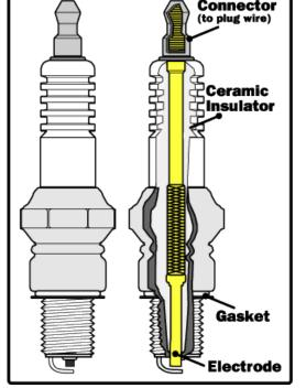
**Spark Plug Cutaway**
